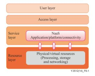
Figure 6-1 – High-level concept of NaaS
