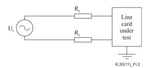
Special test protectors may be used in front of the line card under test if the test is extended to higher voltages.
