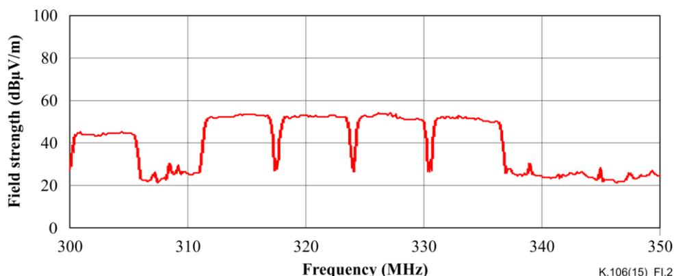
**Figure I.2 – Radio spectrum of disturbance from coaxial cabling**
