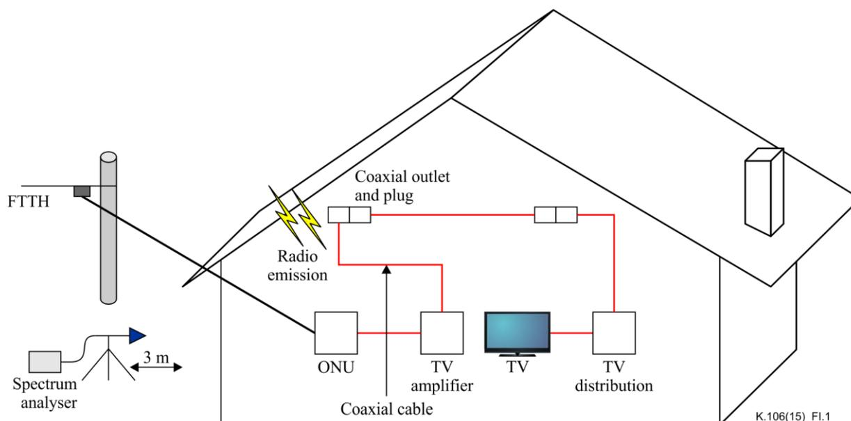
**Figure I.1 – Configuration of telecommunication systems in which a radio disturbance occurred (disturbance caused by TV signal from ONU of FTTH)**
