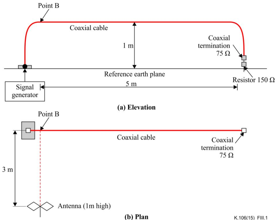
Figure III.1 – Configuration for measurement of emissions from coaxial cables
