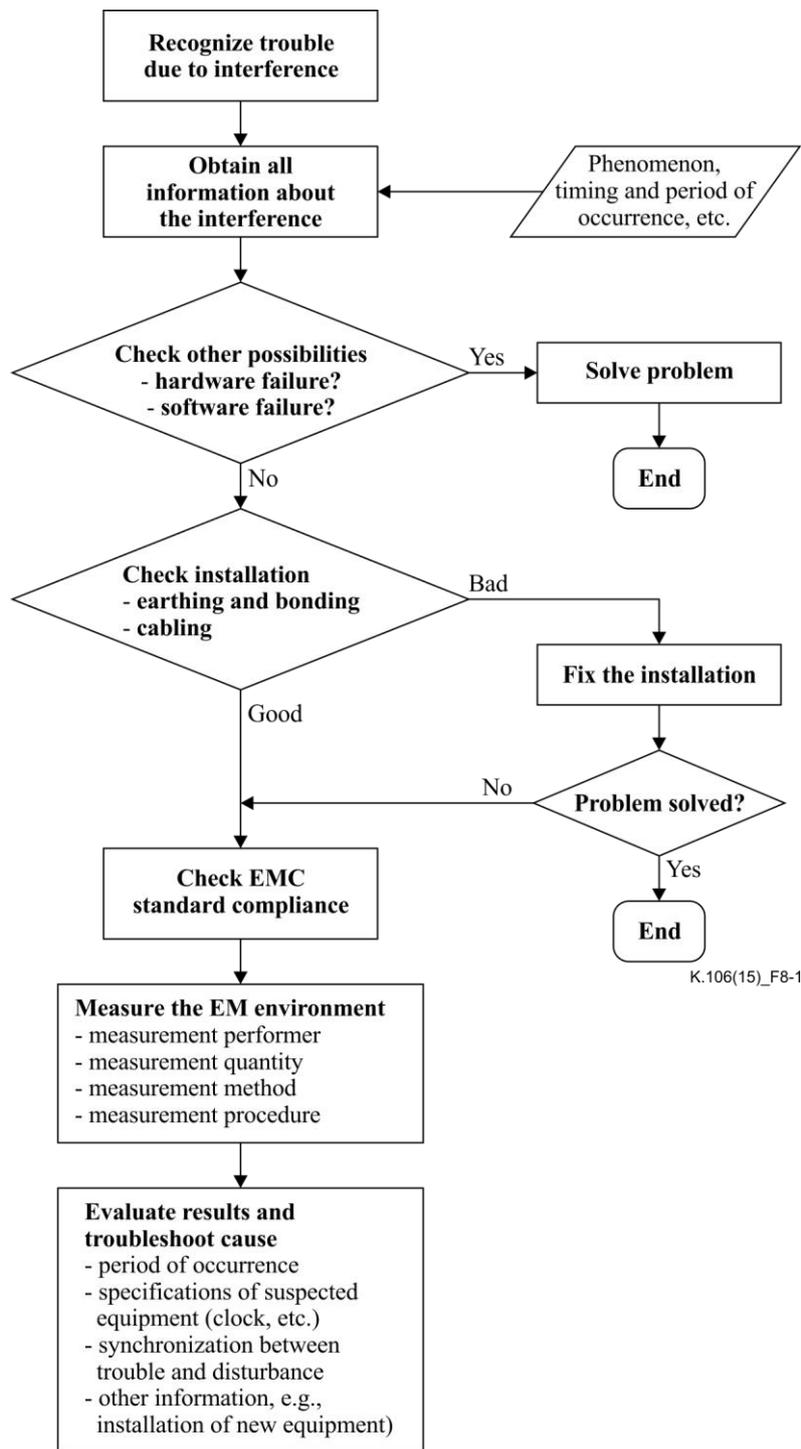
**Figure 8-1 – Interference reduction and troubleshooting flowchart**
