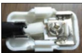
**Figure I.3 – Inferior workmanship at coaxial plug**
