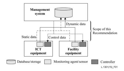
Figure 1 – Architecture of data centre energy management
