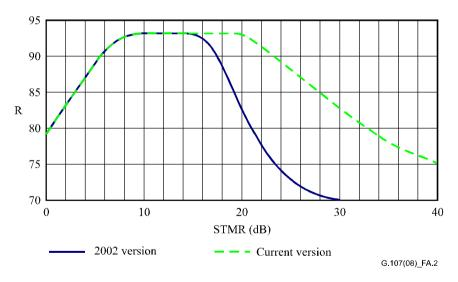
Figure A.2 – Comparison of *R* versus STMR for the current and the previous versions of the E-model algorithm
