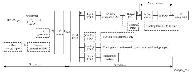
NOTE 1 – Dotted line indicate that the connection is optional. NOTE 2 – Definition of LV should be in accordance with [IEC 60038].
