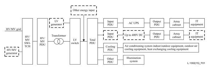
Figure 1 – Example of the architecture of a data centre energy consumption
