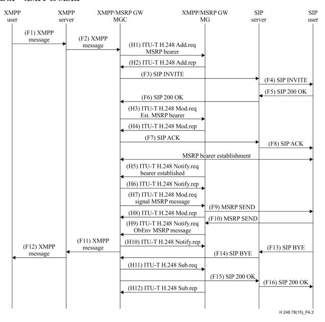
Figure A.2 – XMPP to MSRP order of events in an ITU-T H.248 controlled gateway
