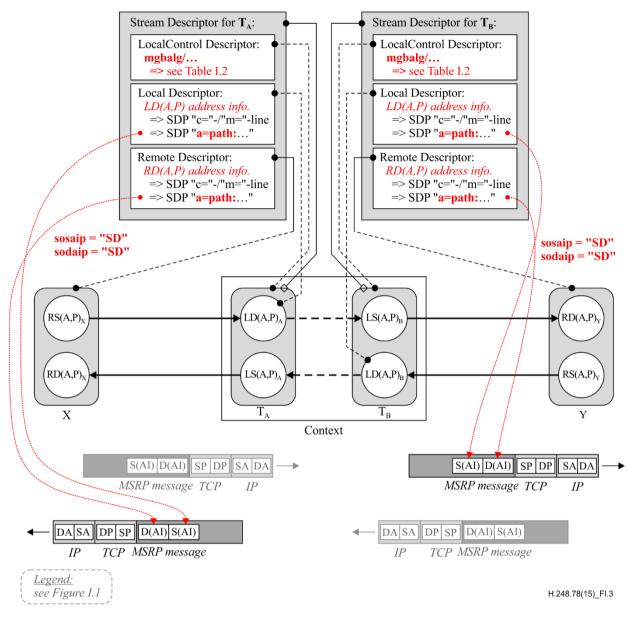
Figure I.3 – Use case "Bidirectional B-ALG with source and destination address information translation" – MSRP bearer traffic
