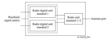
Figure 1 – multi-standard radio base station
