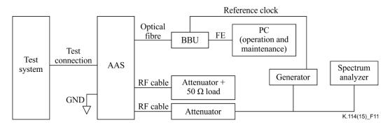
Figure 11 – A typical test configuration for active antenna system base stations
