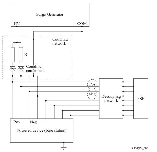
NOTE – For each coupling network, R shall be 80  $\Omega$  with indoor cable and shall be 25  $\Omega$  with outdoor cables.
