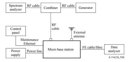
Figure 9 – A typical test configuration for micro base stations
