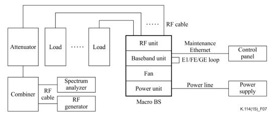
NOTE - E1/FE/GE ports can be connected using a self-test loop or to auxiliary equipment, as long as business functions can be achieved.
