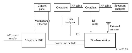
**Figure 10 – A typical test configuration for pico base stations**
