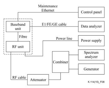
Figure 8 – A typical test configuration for distributed base stations
