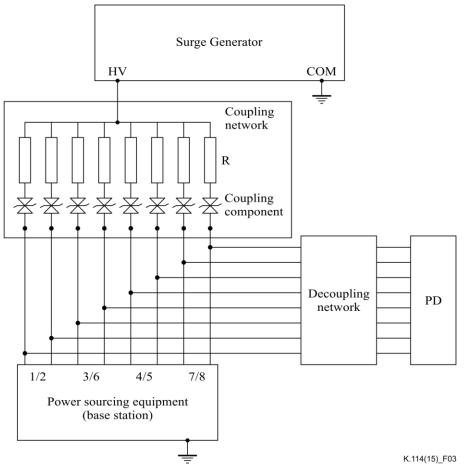
NOTE – For each coupling network, R shall not exceed 250  $\Omega$  with indoor cables and shall be 25  $\Omega$  with outdoor cables.
