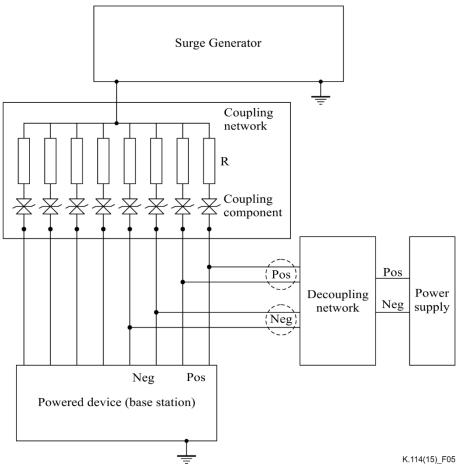
NOTE – For each coupling network, R shall not exceed 250  $\Omega$  with indoor cable and shall be 25  $\Omega$  with outdoor cables.
