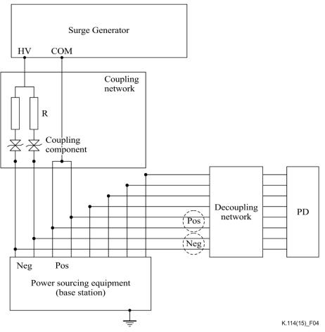
NOTE – For each coupling network, R shall be 80  $\Omega$  with indoor cable and shall be 25  $\Omega$  with outdoor cables.
