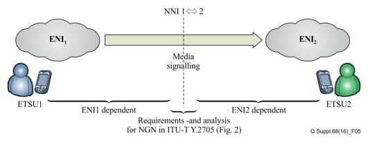
Figure 5 – Security recommendation in the NNI between two ENIs from [ITU-T Y.2705]
