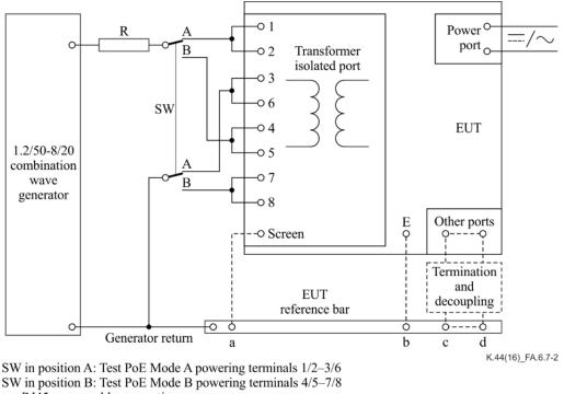
a = RJ45 screen cable connection
