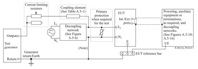
NOTE - Total lead length, per SPD, to connect the primary protection shall be one metre
