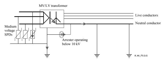
**Figure II.5-5** – **Transfer of overvoltage to neutral**
