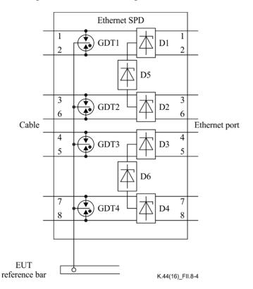
Figure II.8-4 – Block diagram of an Ethernet SPD
