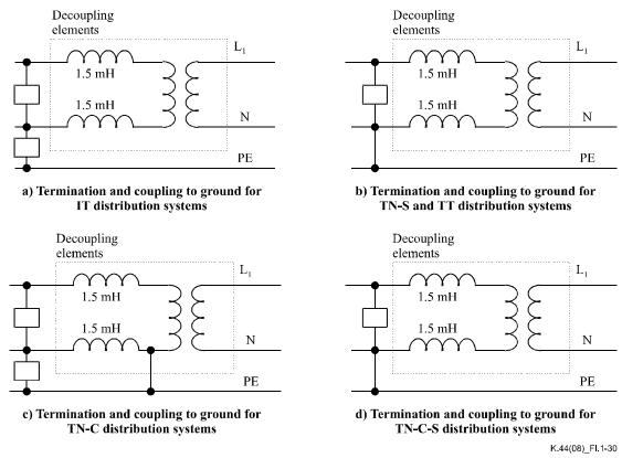
**Figure I.1-30** – **Terminations and coupling to earth for mains ports**
