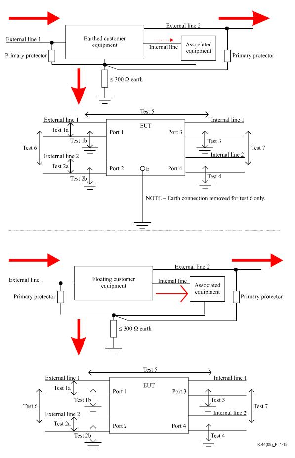
Figure I.1-18 – Scenario for customer equipment
