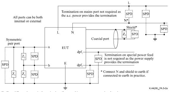
$Z_1$ ,  $Z_2$  and  $Z_3$  are the nominal terminations for a working system or associated equipment. The SPDs are used to couple the required untested port to ground in turn.
