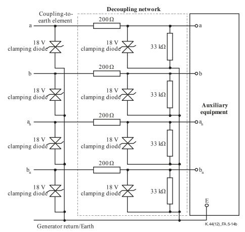
NOTE 1 – Normally, 18 V clamping diodes are used to protect the internal interface. If these diodes prevent normal operation, a diode with a higher clamping voltage may be used. If the 200 ohm decoupling resistor prevents normal operation, a resistor with a lower value may be used.
