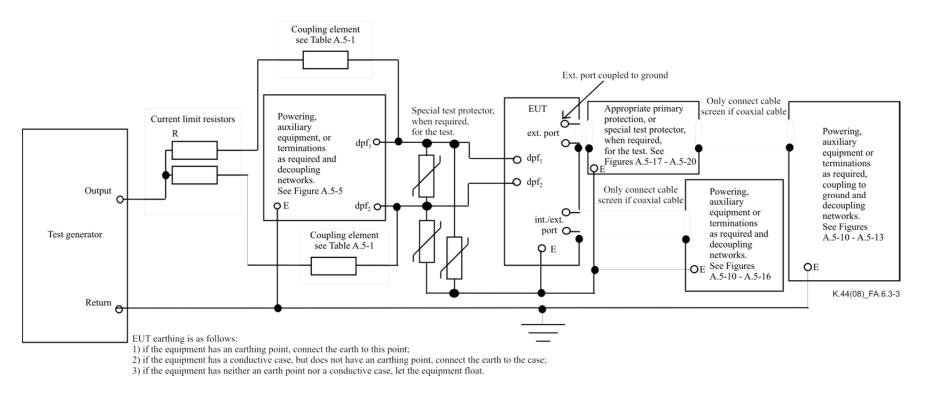
Figure A.6.3-3 – Example of test circuit for an overvoltage or overcurrent on a single external dpf port to external port
