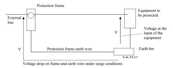
Figure II.3-7 – Voltage drop in earth wires
