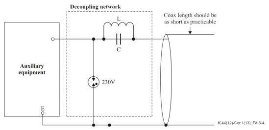
$C > 5 / (2 \times \pi \times f \times Zo)$ , where  $\pi = 3.1416$ , f is the lower frequency used by the EUT and Zo is the characteristic impedance of the coaxial cable. the upper bound to C is 50 nF.
