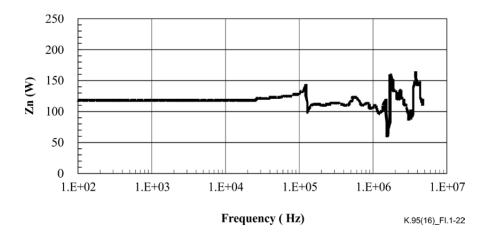
Figure I.1-22 – Normal mode impedance
