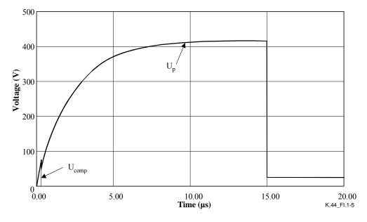
Figure I.1-5 – Voltage  $U_p$  across the special test protector for a charging voltage  $U_c$  of 855 V
