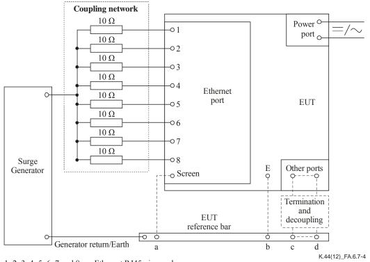
1, 2, 3, 4, 5, 6, 7 and 8 are Ethernet RJ45 pin numbers a = RJ45 screen cable connection b = EUT protective or functional earth connection
