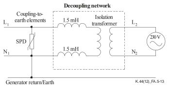
b) Coupling to earth and termination of an untested mains port
