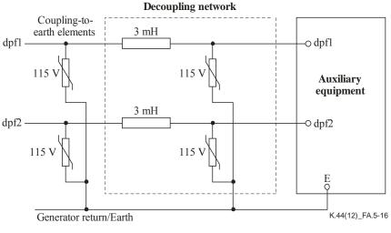
b) Coupling to earth and termination of an untested internal d.c. power port
