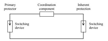
b) Switching device followed by a switching device
