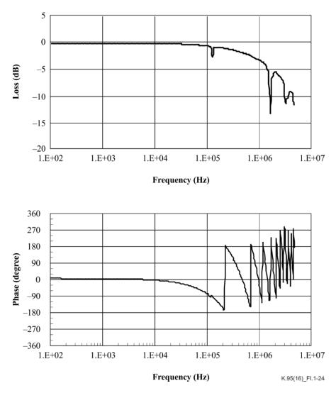
**Figure I.1-24** – **Frequency characteristics of transmission loss**
