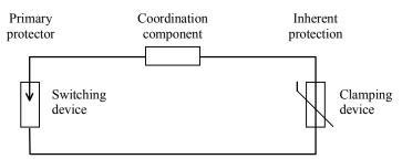
a) Switching device followed by a clamping device
