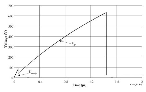
Figure I.1-6 – Voltage  $U_p$  across the special test protector for a charging voltage  $U_c$  of 4 kV
