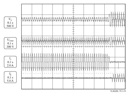
Figure I.1-14 –  $U_{a.c.}$  = 280  $V_{rms}$ , special test protector operating
