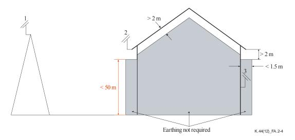
Figure A.2-4 – Classification of antenna ports
