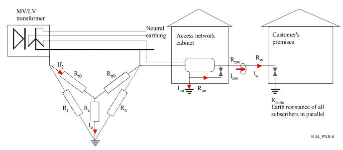
Figure II.5-4 – Mechanism of current flow through equipment
