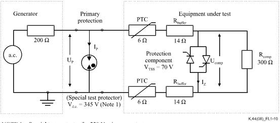
NOTE 1 – Special test protector for 230 V primary protector. NOTE 2 – In practice, the total resistance of  $R_{buffer}$  + the PTC may vary from 10-100  $\Omega$  and  $R_{comp}$  may also have different values.
