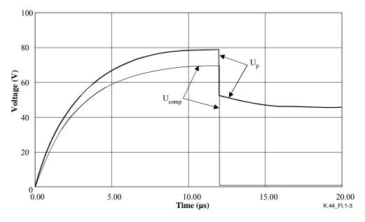
Figure I.1-3 – Voltages with  $U_c$  to give a  $U_{comp}$  of 70 V
