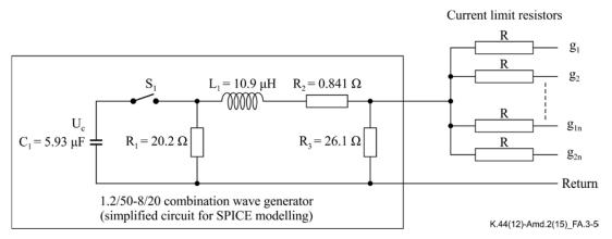
NOTE 1 – The 1.2/50 open-circuit voltage waveshape shall be according to [IEC 60060-1] having a front time of 1.2  $\mu$ s ± 30% and a time to half value from virtual zero of 50  $\mu$ s ± 20%.
