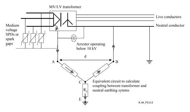
Figure II.5-3 – Limiting EPR by earthing design
