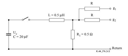
L is small and mostly parasitic inductance of the wiring, may need to be adjusted to give the required front time of 2  $\mu$ s. U<sub>c</sub> is adjusted to give required o/c output voltage.
