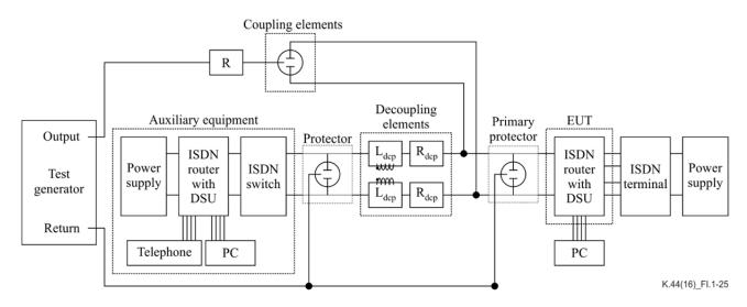
Figure I.1-25 – Test set-up for ISDN equipment
