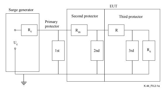
Figure II.2-1a – Principle of protection by ladder circuits
