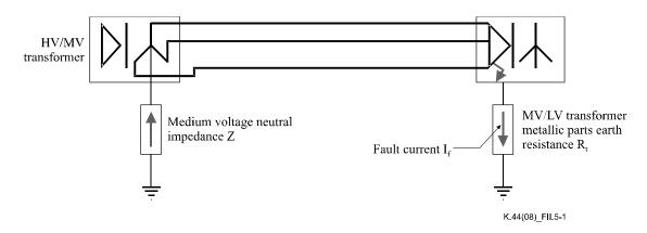
Figure II.5-1 – Factors affecting the fault current
