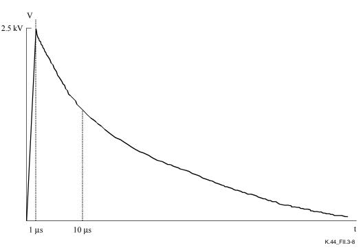
Figure II.3-8 – Earth voltage drop
