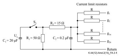
NOTE 1 – The 10/700 open-circuit voltage waveshape shall have a front time of 10  $\mu$ s ±3  $\mu$ s and a time to half value from virtual zero of 700  $\mu$ s ±144  $\mu$ s.
