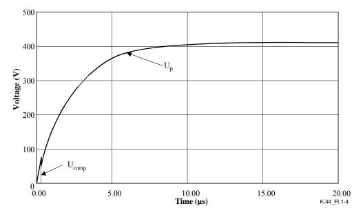
Figure I.1-4 – Voltages with  $U_c$  set to cause a  $U_p$  just below the sparkover voltage of the GDT
