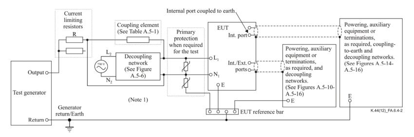
NOTE 1 - Total lead length, per SPD, to connect the primary protection shall be one metre
