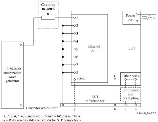
a = RJ45 screen cable connection for STP connection b = EUT protective or functional earth connection c to d = Terminals of all other signal ports
