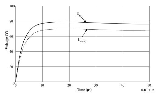
Figure I.1-2 – Voltages with  $U_c$  to give a  $U_{comp}$  of 69 V
