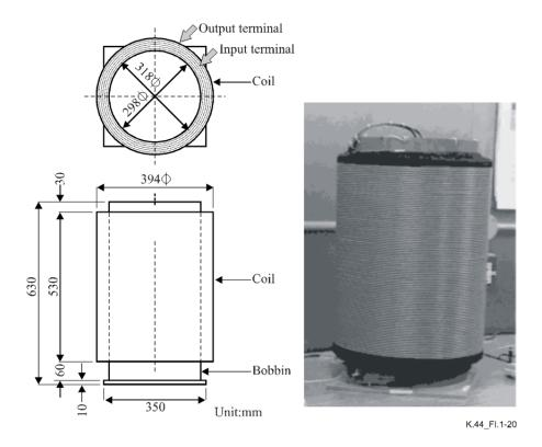
Figure I.1-20 – Configuration, size and overview of 20 mH coil
