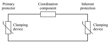
c) Clamping device followed by a clamping device
