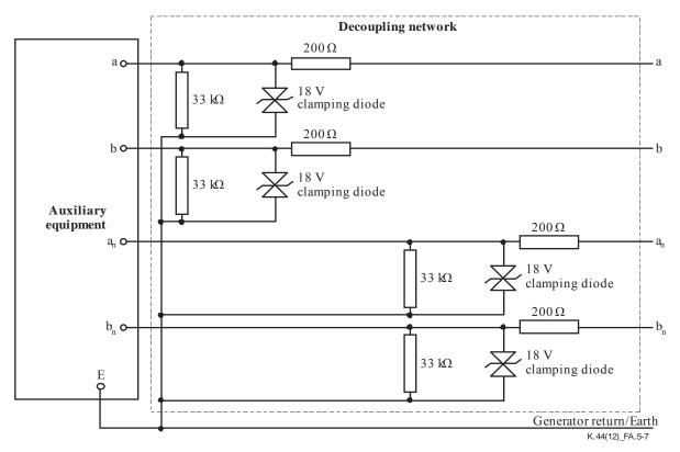
NOTE – Normally, 18 V clamping diodes are used to protect the internal interface. If these diodes prevent normal operation, a diode with a higher clamping voltage may be used. If the 200 ohm decoupling resistor prevents normal operation, a resistor with a lower value may be used.
