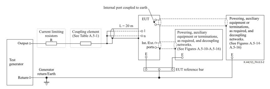
For repeatability of measurement, it is recommended that the test be performed on an earth reference plane, with the cable laid on the ground plane in a snake pattern. All conductors are connected together and with the shield. (Reason: in worst case, inserted protective elements in the auxiliary equipment – not included in this test set-up – can cause short circuit termination.)
