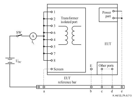
$$\begin{split} U_{DC} &= DC \text{ test voltage (limited to 100 mA)} \\ SW &= Switch closed for current measurement} \\ A &= A \text{ meter used to measure leakage current, } I_L \\ Insulation resistance &= U_{DC}/I_L \end{split}$$
