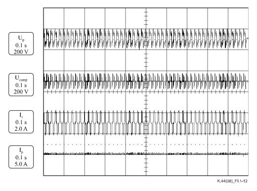
Figure I.1-12 –  $U_{a.c.} = 200 V_{rms}$ , switching inherent protector operating, but not PTC
