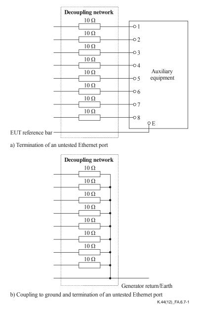
Figure A.6.7-1 – Termination and coupling to earth of untested Ethernet ports
