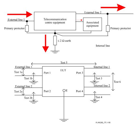
Figure I.1-16 – Test conditions for telecommunication centre equipment
