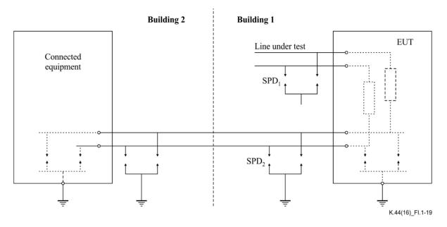
**Figure I.1-19 – Terminations and SPDs on equipment**
