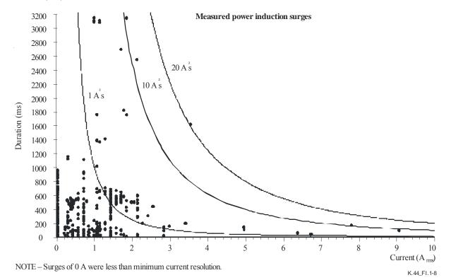
Figure I.1-8 – Power induction overcurrents measured in Australia
