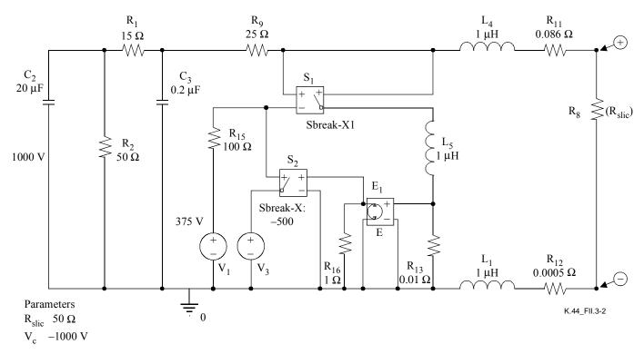
Figure II.3-2 – The Spice model used to calculate the reduced voltage at the equipment input due to the impedance of the MDF cable
