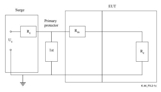
Figure II.2-1c – Robust circuits with no second protector
