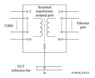
Figure II.8-3 – In-line screened transformer isolation
