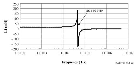
Figure I.1-23 – Frequency characteristics of inductance
