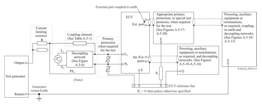
NOTE - Total lead length, per SPD, to connect the primary protection shall be one metre
