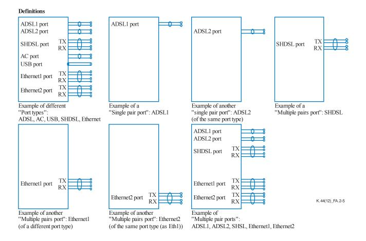
Figure A.2-5 – Examples of equipment ports
