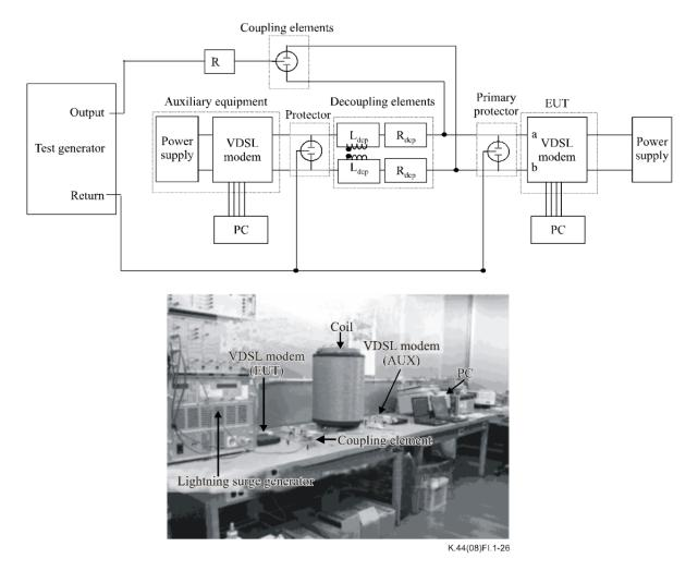
Figure I.1-26 – Test set-up for VDSL equipment
