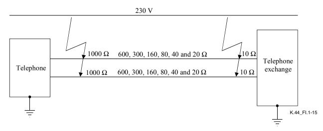
Figure I.1-15 – Mains power contact mechanism
