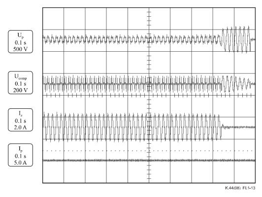
$\label{eq:Figure I.1-13-U_{a.c.}=220 V_{rms}, PTC \ operates \ at \ end \ of \ test \ (2 \ s),} \\ below \ firing \ voltage \ of \ special \ test \ protector$
