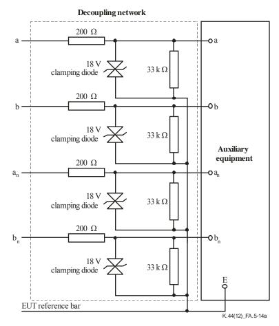
NOTE 1 – Normally, 18 V clamping diodes are used to protect the internal interface. If these diodes prevent normal operation, a diode with a higher clamping voltage may be used. If the 200 ohm decoupling resistor prevents normal operation, a resistor with a lower value may be used.
