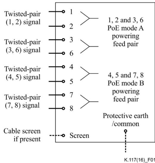
**Figure 1 – Ethernet RJ45 contact connections**
