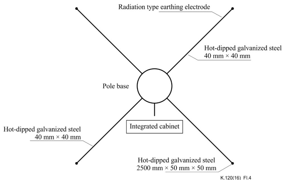
**Figure I.4 – Earth electrodes for an MBS installed on a street light**
