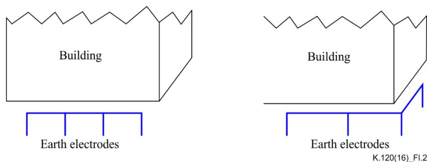
**Figure I.2 – Earth electrodes for an MBS installed on the external wall of an existing building**
