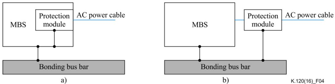
**Figure 4 – Protection module on AC power cable**
