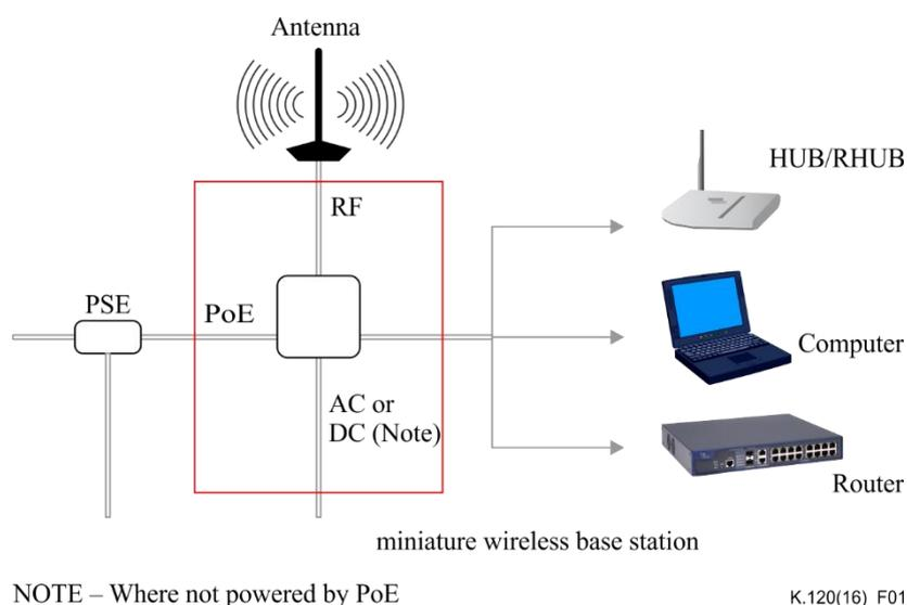
**Figure 1 – Typical configuration of miniature wireless base system**
