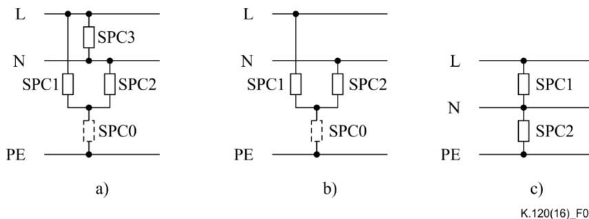
NOTE – Where SPC0 exists in Figures 5a and 5b, its nominal discharge current shall be twice the value specified in Table 1.
