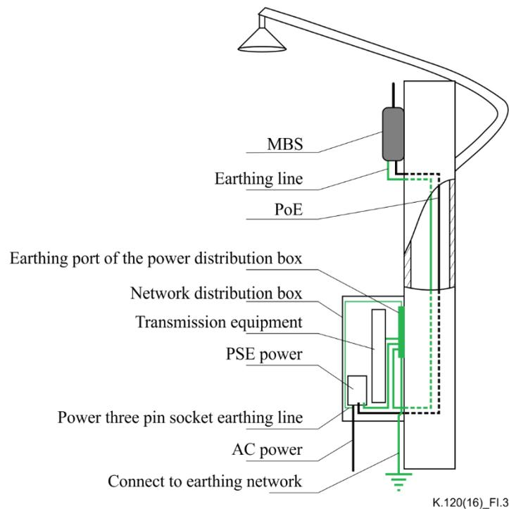
**Figure I.3 – MBS installed on a street light**
