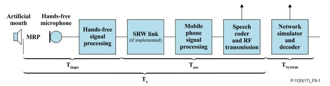
Figure 9-1 – Different blocks contributing to the delay in send direction
