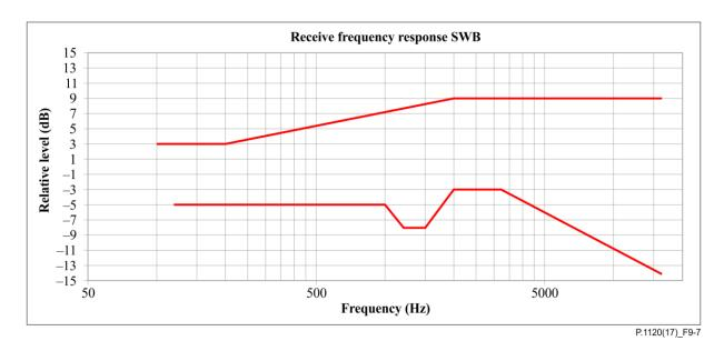
Figure 9-7 – Tolerance mask for the SWB headset receive sensitivity frequency response (Figure is informative)
