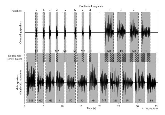
Figure 9-14 – Double talk test sequence with overlapping speech sequences in receive and send directions
