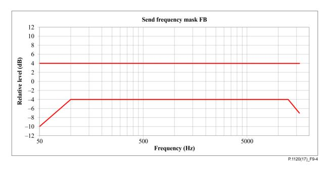
Figure 9-4 – Tolerance mask for the FB send sensitivity frequency response (Figure is informative)
