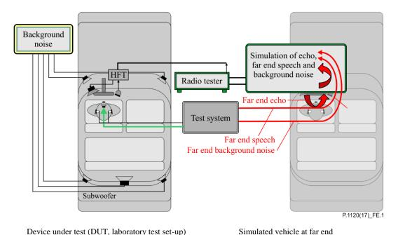
Figure E.1 – Test set-up for simulating insufficient far-end echo loss
