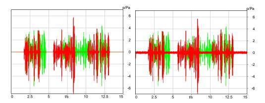
The transmitted speech signals are recorded in receive direction of the DUT, i.e., in the vehicle in the laboratory set-up. No howling or feedback shall be detected.
