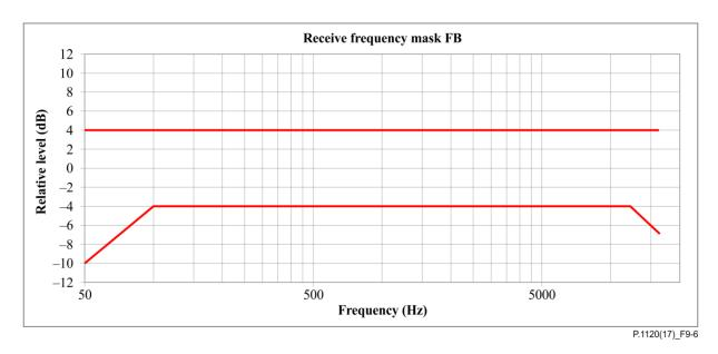
Figure 9-6 – Tolerance mask for the FB receive sensitivity frequency response (Figure is informative)
