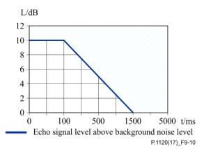
Figure 9-10 – Initial convergence with background noise, requirement on echo signal level vs time
