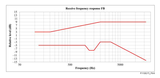
Figure 9-8 – Tolerance mask for the FB headset receive sensitivity frequency response (Figure is informative)
