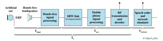
Figure 9-2 – Different blocks contributing to the delay in receive direction
