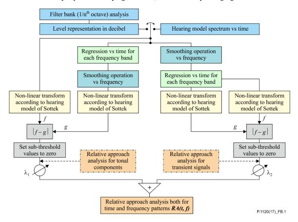
Figure B.1 – Block diagram of Relative Approach
