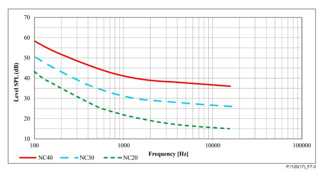
Figure 7-3 – NC-criteria for test environment (values above 8 kHz extrapolated)
