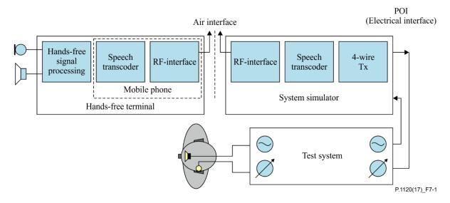
Figure 7-1 – Test arrangement for hands-free terminal
