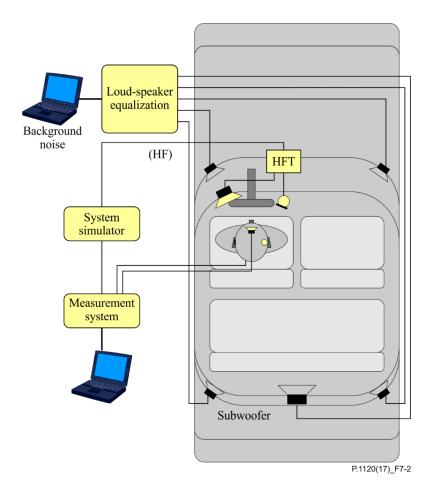
Figure 7-2 – Test arrangement with background noise simulation
