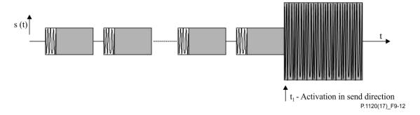
Figure 9-12 – Structure of the test signal for measuring the attenuation range
