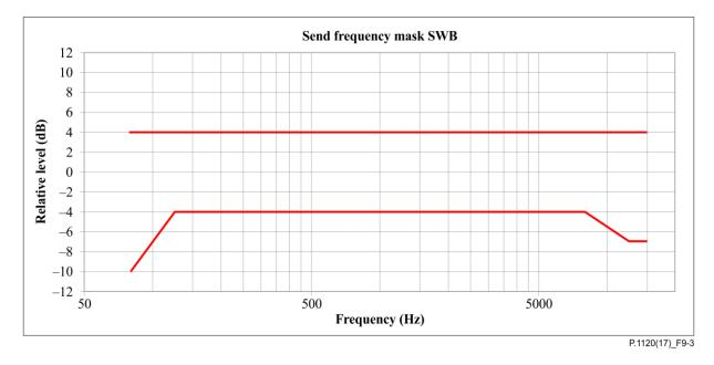
Figure 9-3 – Tolerance mask for the SWB send sensitivity frequency response (Figure is informative)
