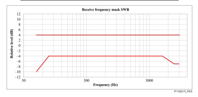
Figure 9-5 – Tolerance mask for the SWB receive sensitivity frequency response (Figure is informative)
