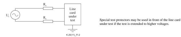
Figure I.2 – Test set-up for floating power induction and earth potential rise
