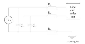
Coupling resistors,  $R_c$ , represent the line resistances; capacitances,  $C_c$ , represent the line capacitances to earth and  $R_c$  represents the earthing resistance of the overvoltage protectors at the subscriber end of the line.
