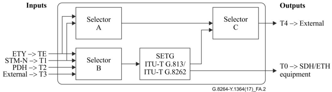
**Figure A.2 – Hybrid SDH/synchronous Ethernet SETS function**
