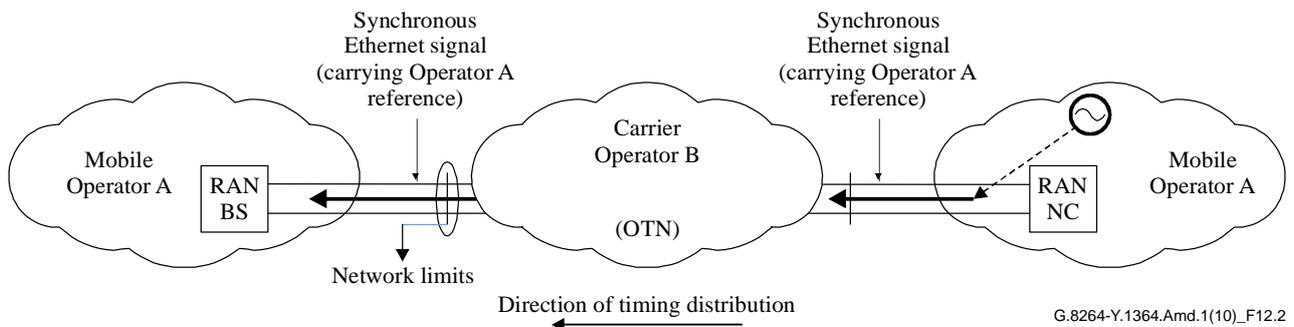
**Figure 12-2 – Illustration of a timing transparent transport of the synchronous Ethernet client signals in the multi-operator context**
