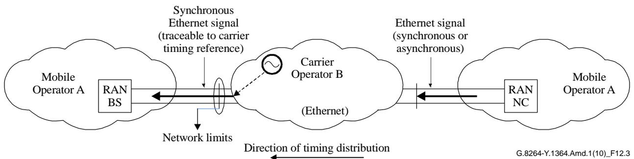
**Figure 12-3 – Illustration of a synchronous Ethernet synchronization service in the multi-operator context**
