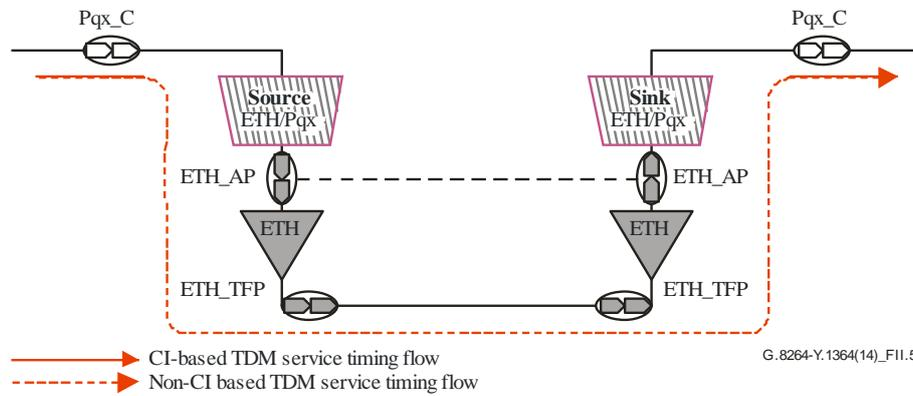
**Figure II.5 – Functional models for adaptive timing**
