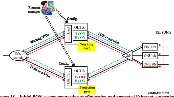
Figure 18 – Initial PON system connection configuration and protected Ethernet connections with two associated VLAN identifiers
