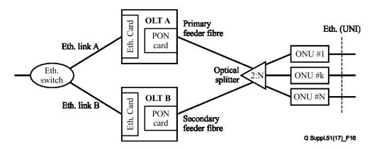
Figure 16 – General physical configuration of a dual-parented type B PON protection
