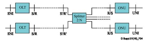
Figure 4 – Dual-parented type B protection
