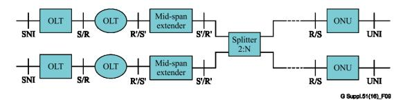
Figure 9 – Extended type B protection architecture with two independent reach extender units
