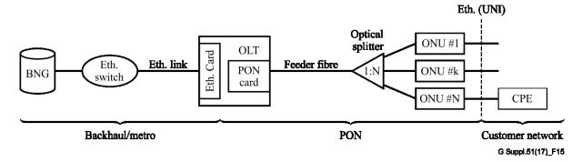
Figure 15 – Elements of a connection between a CPE and BNG over a PON and backhaul
