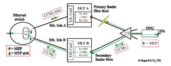
Figure 20 – Ethernet linear protection at a glance
