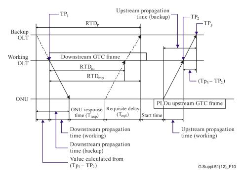
Figure 10 – Relationship between time references when the backup path is longer than the working path
