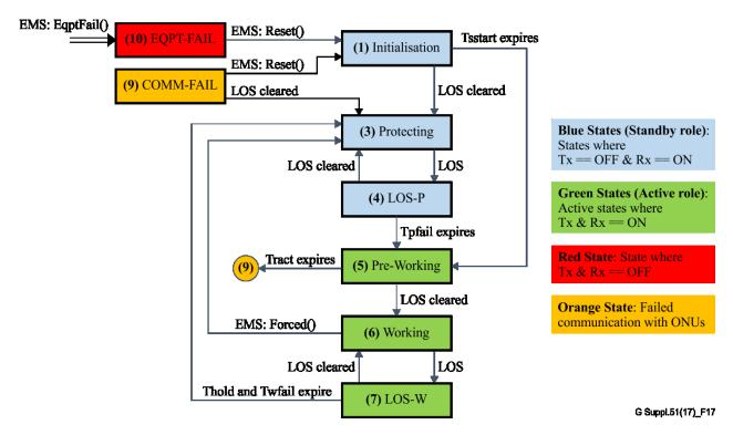
Figure 17 – OLT port state machine diagram
