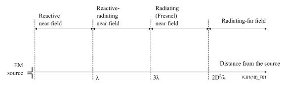
Figure 1 – Field regions around an EM source (the antenna maximum dimension D is supposed to be large compared with the wavelength  $\lambda$ )
