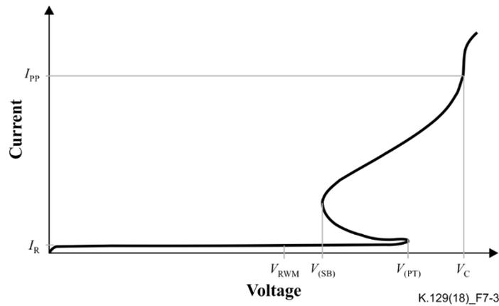
**Figure 7-3 – Punch-through diode and fold-back diode characteristic**
