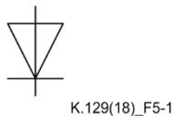
**Figure 5-1 – Semiconductor diode, general symbol (symbol S00641)**
