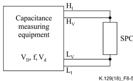
**Figure 8-5 – Kelvin connected capacitance measurement**
