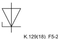
**Figure 5-2 – Breakdown diode, unidirectional (symbol S00646)**
