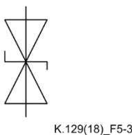
**Figure 5-3 – Breakdown diode, bidirectional (symbol S00647)**
