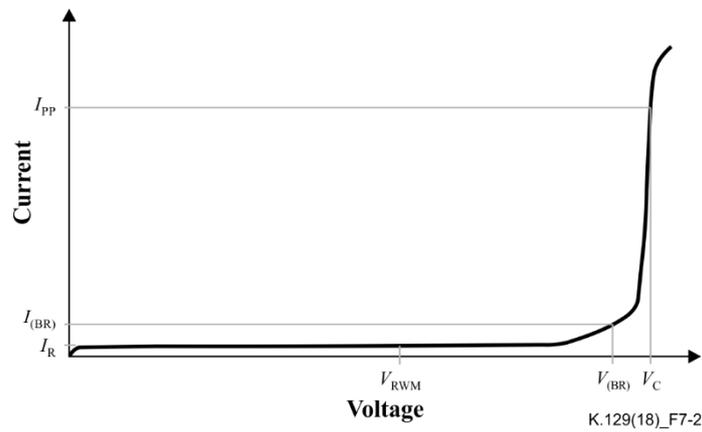
**Figure 7-2 – Breakdown diode characteristic**
