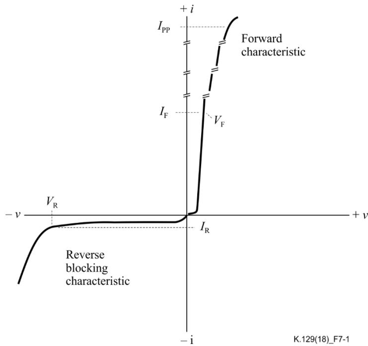
**Figure 7-1 – Diode characteristic**
