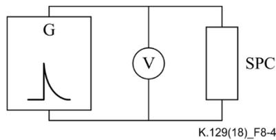
**Figure 8-4 – Surge verification and voltage measurement circuit**
