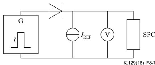
**Figure 8-7 – Transient thermal impedance test circuit**
