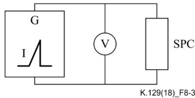
**Figure 8-3 – Current ramp, voltage measurement circuit**
