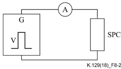
**Figure 8-2 – Voltage pulse, current measurement circuit**
