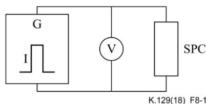
Figure 8-1 – Current pulse, voltage measurement circuit
