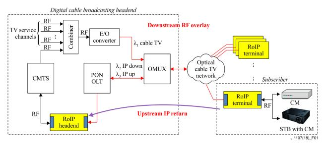
Figure 1 – System architecture for radio over Internet protocol
