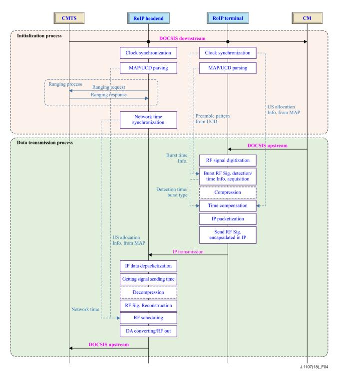
Figure 4 – Service flow of radio over Internet protocol service
