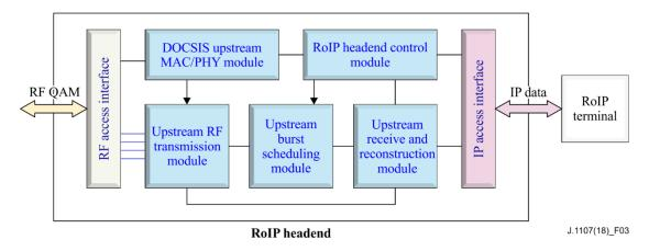
Figure 3 – Architecture for radio over Internet protocol headend
