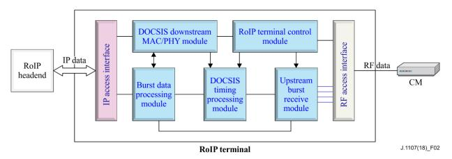
Figure 2 – Architecture for radio over Internet protocol terminal
