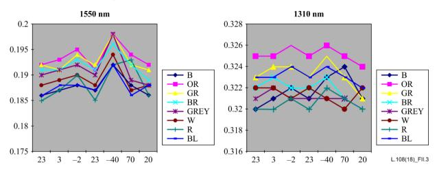
Figure II.3 – Largest attenuation values in each loose tube at different temperature points
