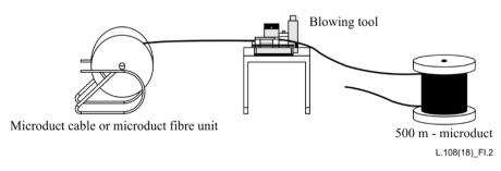
Figure I.2 – Test set-up for blowing performance on drum
