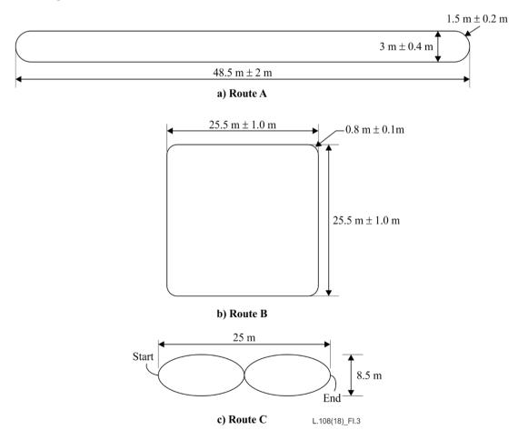
Figure I.3 – Test set-up for blowing performance in the field (simulated)
