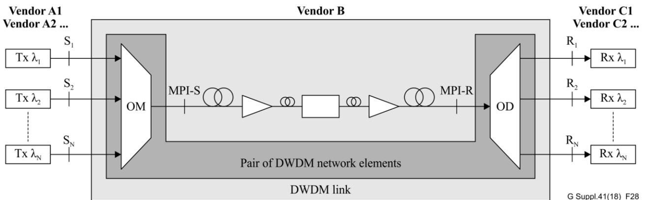
**Figure 28 – Multi-span black-link transverse compatibility**
