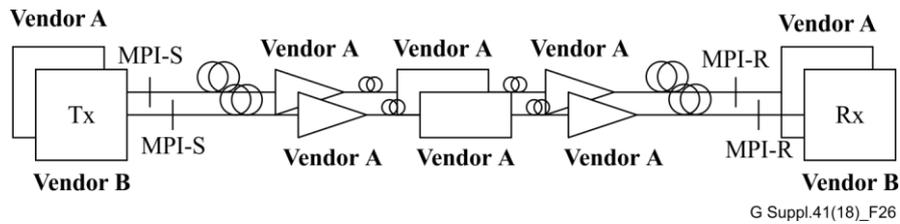
**Figure 26 – Multi-span black-box multiple-link transverse compatibility**
