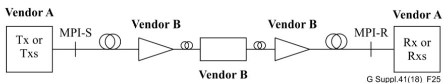
**Figure 25 – Multi-span black-box single-link transverse compatibility**
