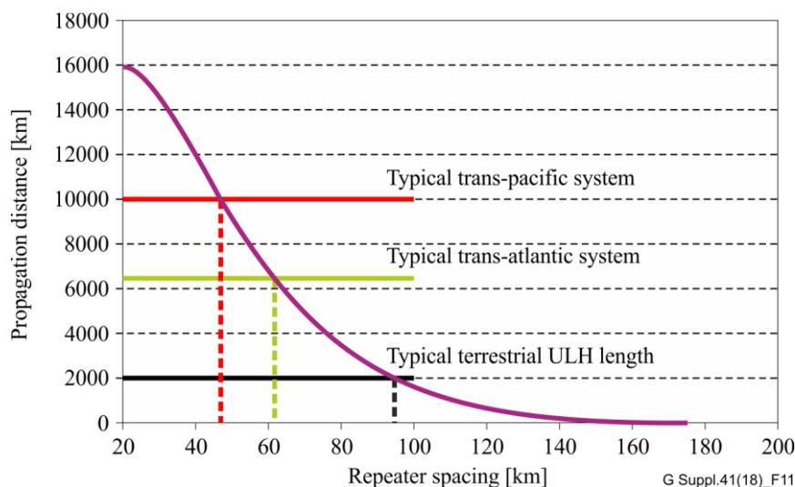
NOTE – The parameters used are: OSNR = 16 dB in a reference bandwidth  $B_r = 0.1$  nm,  $NF = 4.7$  dB,  $N_{\lambda} = 64$  channels,  $P_{out} = 14$  dBm and fibre attenuation  $\alpha = 0.21$  dB/km.
