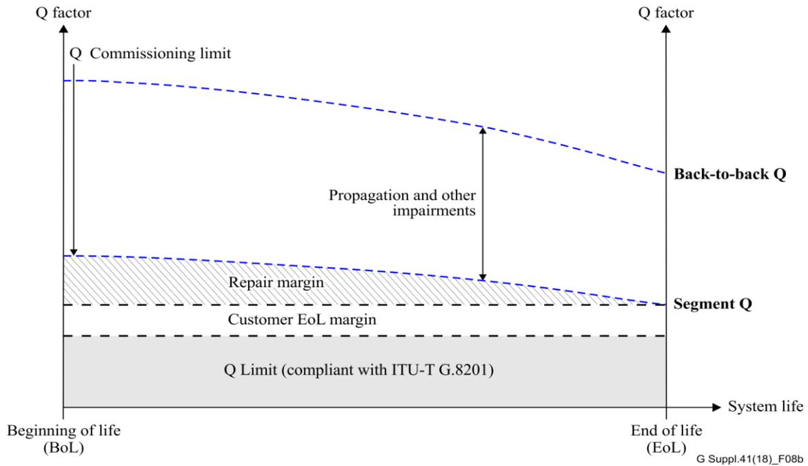
**Figure 8-b – Power budget structure of example 2**
