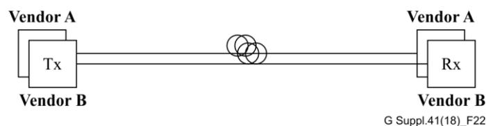
**Figure 22 – Single-span longitudinal compatibility**
