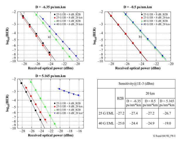
Figure 8-3 – 25 Gbit/s and 40 Gbit/s EML dispersion penalty comparison after 20 km (a) in O- band, (b) in zero dispersion band and (c) in O+ band
