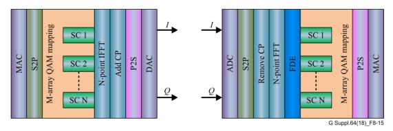
Figure 8-15 – Basic OFDM system architecture
