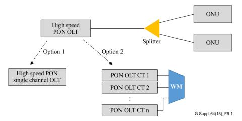
Figure 6-1 – High speed PON architecture
