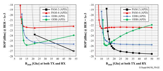
Figure 8-22 – Effect of TX/RX frequency response, comparison of Butterworth (left) and S-Gaussian (right) filter models, varying B<sub>20dB</sub>
