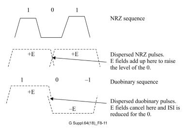
Figure 8-11 – ODB interference offset to avoid ISI
