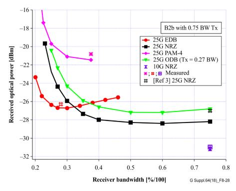
Figure 8-28 – Back-to-back experiment results, ER = 13 dB (5.5 dB PAM-4). TX filter response –3 dB point at 0.75 x bit rate for NRZ and EDB, 0.27 × bitrate for ODB, 0.75 × baud rate (0.375 × bit rate) for PAM-4
