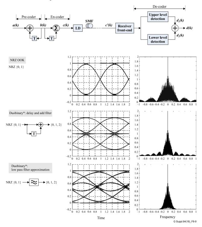
Figure 8-9 – Coding and decoding schematic diagram of EDB
