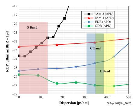
Figure 8-25 – Effect of chromatic dispersion, two-pole Butterworth TX/RX response, B<sub>3dB</sub>=7 GHz
