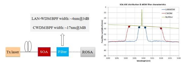
Figure 8-33 – SOA spectrum after narrow band pass filters
