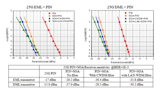
Figure 8-34 – 25 Gbit/s PIN+SOA receiver performance on EML and DML signal
