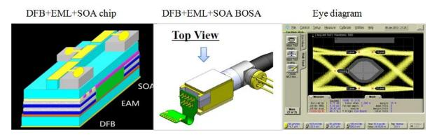
Figure 8-32 - Schematic of EML transmitter with SOA integrated on the laser chip
