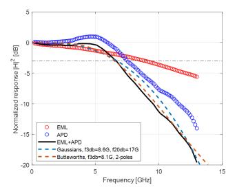
Figure 8-24 – Comparison between the filter model and the experimental data from the JLT paper mentioned in the text
