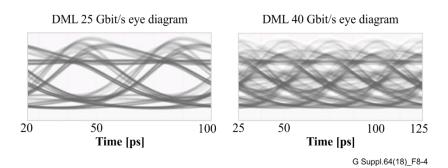
Figure 8-4 - Simulated eye diagram of DML laser with 25 Gbit/s and 40 G NRZ modulation
