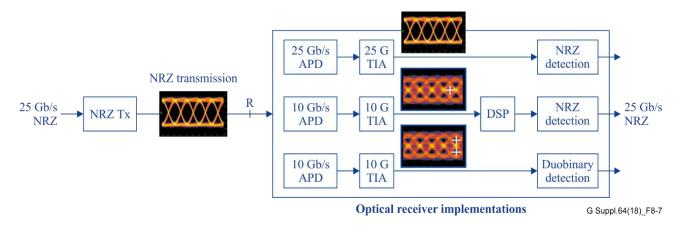
Figure 8-7 – NRZ transmission and multiple receiver implementation options
