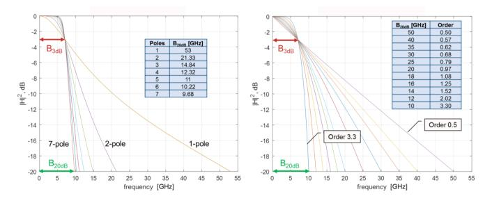
Figure 8-20 – 3 dB and 20 dB bandwidths for Butterworth (left) and S-Gaussian (right) filters
