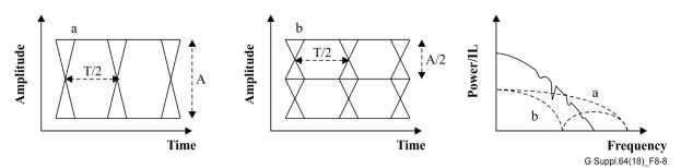
Figure 8-8 – Schematic of NRZ waveform (left), EDB waveform (middle) and the corresponding power spectrum diagram (right)
