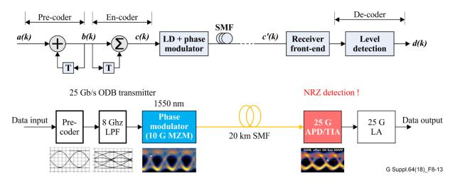
Figure 8-13 – Coding and decoding schematic diagram of 25 Gbit/s ODB
