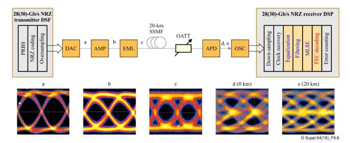
Figure 8-6 – Schematic of the 28-Gbit/s NRZ-DSP equalization experiment set-up. (a-e): measured eye diagrams at different locations in the transmission link
