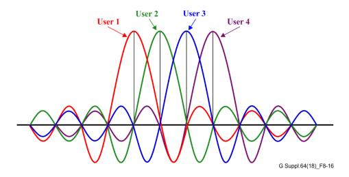
Figure 8-16 – Frequency-domain OFDM subcarrier multiplexing for multi-user access
