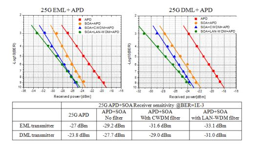
Figure 8-35 – 25 Gbit/s APD+SOA receiver performance on EML and DML signal
