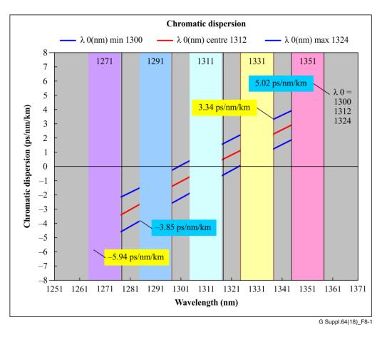
Figure 8-1 – Chromatic dispersion coefficient of ITU-T G.652 fibre in O-band
