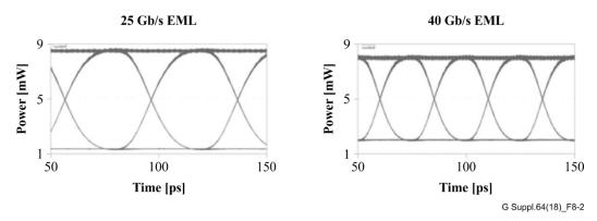
Figure 8-2 – Simulated eye diagram of EML laser with 25 Gbit/s and 40G NRZ modulation
