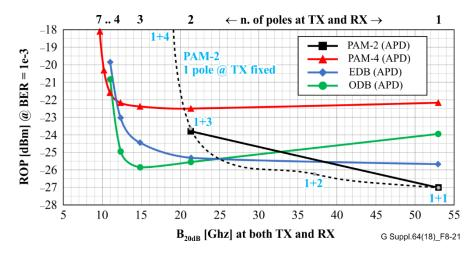
Figure 8-21 – Effect of TX/RX frequency response, Butterworth filter model, varying B<sub>20dB</sub> (number of poles); the dashed line represents the case with a single-pole TX and a varying number of poles at RX
