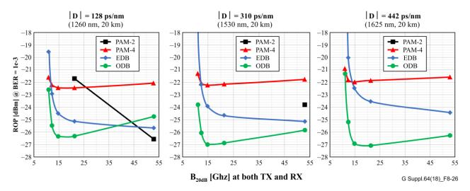
Figure 8-26 – Effect of dispersion and TX/RX frequency response, Butterworth filter model, B<sub>3dB</sub>=7 GHz, varying B<sub>20dB</sub> and |D|
