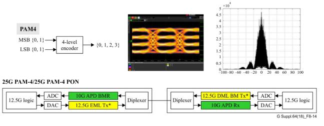
Figure 8-14 – Schematic of PAM4 modulation
