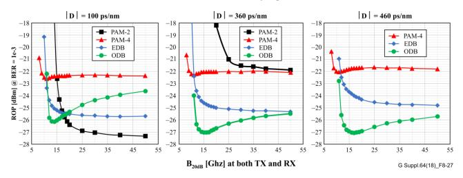
Figure 8-27 – Effect of dispersion and TX/RX frequency response, S-Gaussian filter model, B<sub>3dB</sub>=7 GHz, varying B<sub>20dB</sub> and |D| (note: |D| values are not the same of Figure 8-25)
