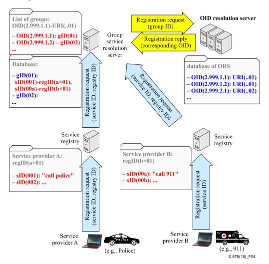
**Figure 4 – Service and OID registration procedure**
