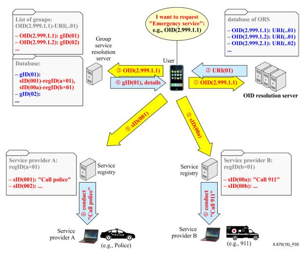
Figure 5 – OID-based resolution procedure for a group of IoT services
