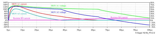
Figure IV.2-2 – SPICE circuit MOV A1 and A3 voltage and current with a floating supply (R7 = 10 M $\Omega$  and R8 = 10 M $\Omega$ ), a 100 m connecting cable and the powered equipment port represented as a resistor (R9 = 10  $\Omega$ )
