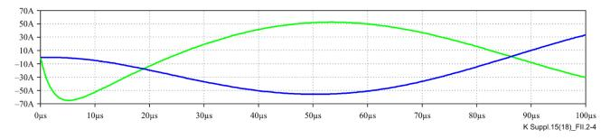
Figure II.2-4 – SPICE circuit port current waveforms with an earth bonded supply (R7 = 0 and R8 = 10 M $\Omega$ ), a 1 m connecting cable and the powered equipment port represented by a capacitor (C4 = 100  $\mu$ F)
