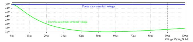
Figure II.2-2 – SPICE circuit voltage waveforms with an earth bonded supply (R7 = 0 and  $R8 = 10 \text{ M}\Omega$ ), a 100 m connecting cable and the powered equipment port is represented by a capacitor ( $C4 = 100 \ \mu F$ )
