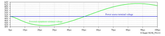
Figure II.2-3 – SPICE circuit voltage waveforms with an earth bonded supply (R7 = 0 and  $R8 = 10 \text{ M}\Omega$ ), a 1 m connecting cable and the powered equipment port represented by a capacitor ( $C4 = 100 \ \mu\text{F}$ )
