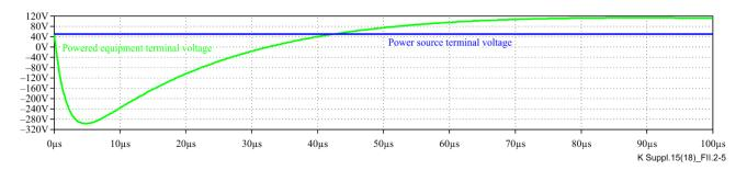
Figure II.2-5 – SPICE circuit port voltage waveforms with an earth bonded supply (R7 = 0 and R8 = 10 M $\Omega$ ), a 100 m connecting cable and the powered equipment port represented as a resistor (R9 = 10  $\Omega$ )
