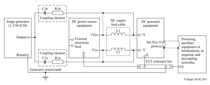
Figure 1 – Example of a common-mode surge test circuit
