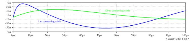
Figure II.2-7 – SPICE circuit connecting cable current waveforms for earth bonding at the powered equipment and the surge applied to the power source DC port with connecting cable lengths of 1 m and 100 m
