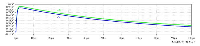
Figure I.2-1 – SPICE circuit waveforms with a floating supply ( $R7 = R8 = 10 M\Omega$ ) with the powered equipment port represented as a capacitor ( $C4 = 100 \mu F$ )
