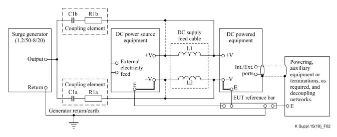
Figure 2 – Example of a test circuit where the applied common-mode surge is converted into a differential surge by equipment earth bonding
