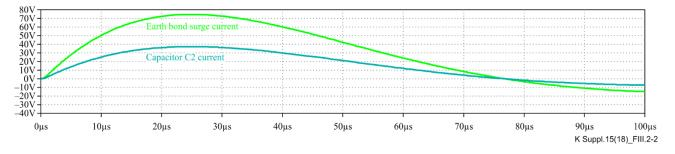
Figure III.2-2 – SPICE circuit powered equipment current waveforms with an earth bonded power sourcing equipment (R7 = 10 M $\Omega$  and R8 = 0), a 100 m connecting cable and the powered equipment port represented as a capacitor (C4 = 100  $\mu$ F)
