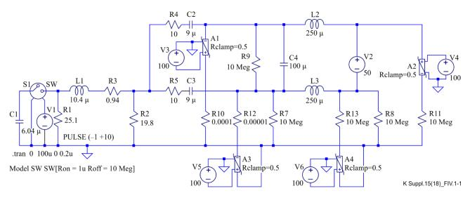
Figure IV.1-1 – Example SPICE DC Interface circuit with four MOV functions added
