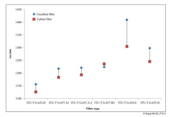
Figure VII.3 – Comparison of λ<sub>cc</sub> on cabled/uncabled fibres (Cable A, stranded loose tube type)
