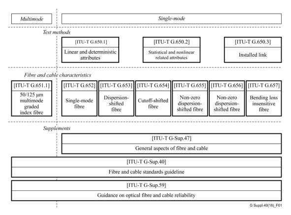
Figure 1 – Relationships amongst Recommendations and supplements related to optical fibres and cables
