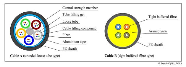
Figure VII.1 – Structure of cable samples: Cable A, 30-fibres stranded loose tube outdoor cable; Cable B, 4-fibres indoor cable
