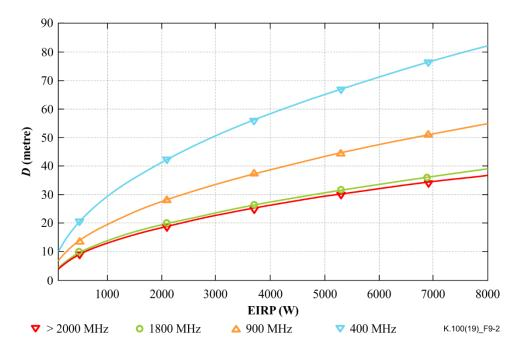
Figure 9-2 – Side length of the assessment domain boundary as a function of the equivalent isotropically radiated power for some frequencies, estimated using equation  $9-1^{13}$
