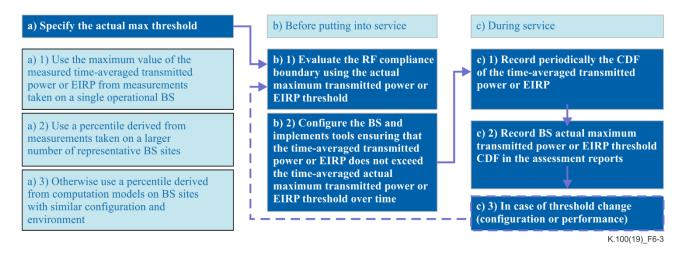
Figure 6-3 – Flow chart for assessing compliance for a BS site sector or sub-division of a BS site sector [b-IEC TR 62669]
