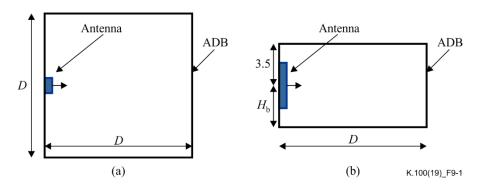
Figure 9-1 – a) Top-view of the square-shaped assessment domain boundary (ADB) with side length D.
