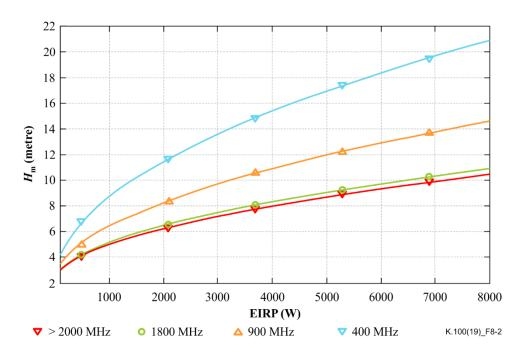
Figure 8-2 –  $H_{\rm m}$  as a function of the equivalent isotropically radiated power obtained from Equations 8-1 to 8-3 based on a conservative choice of antenna parameters:  $\pi/12$  half-power beamwidth  $(\theta_{\rm bw})$ ,  $\pi/12$  antenna downtilt  $(\alpha$ , electrical and mechanical) and side lobe suppression  $(A_{\rm sl})$  of 0.05.  $H_{\rm m}$  will decrease by decreasing  $\theta_{\rm bw}$ ,  $\alpha$  and the side lobe suppression
