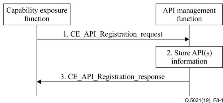
**Figure 8-1 – API registration procedure**
