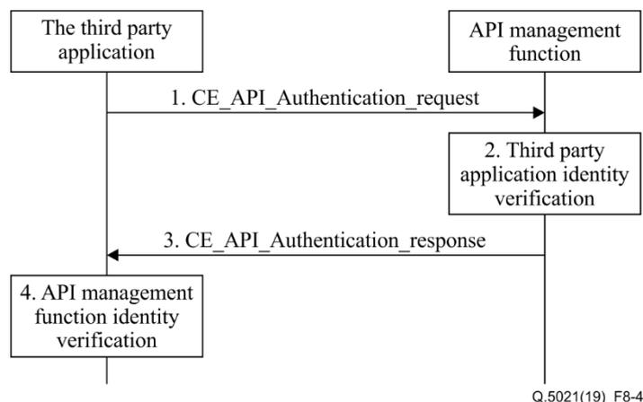
**Figure 8-4 – API authentication procedure**
