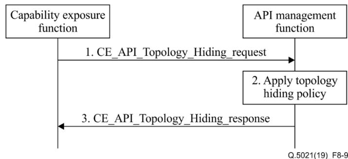
**Figure 8-9 – Topology hiding procedure**
