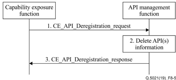
**Figure 8-5 – API deregistration procedure**
