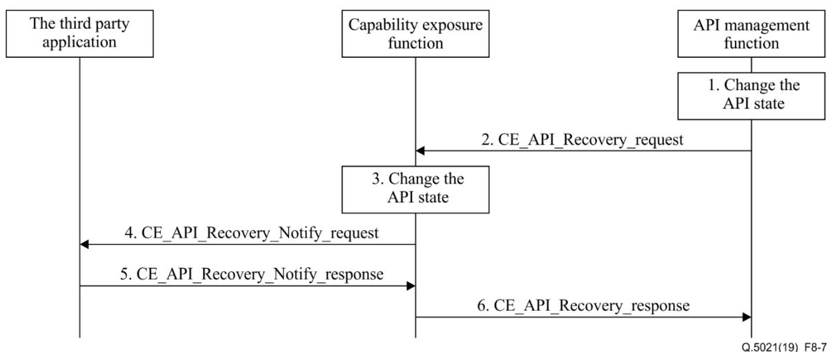
**Figure 8-7 – API recovery procedure**
