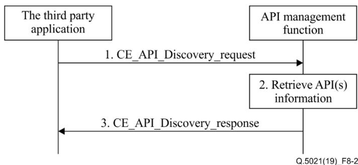
**Figure 8-2 – API discovery procedure**
