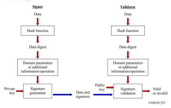
Figure 1 – Digital signature generation and validation
