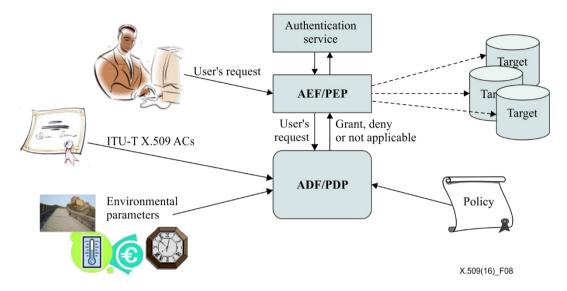
Figure 8 - The control model for a single domain PMI
