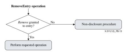
Figure B.13 – Remove Entry operation
