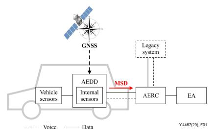
Figure 1 – MSD transmission [ITU-T Y.4119]
