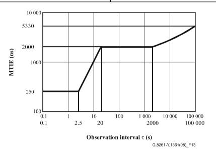
Figure 13 – Network limit for wander (MTIE) at synchronous equipment clock Option 1 interfaces
