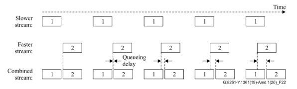
Figure <u>21-22</u> – Beating between regular rate packet streams
