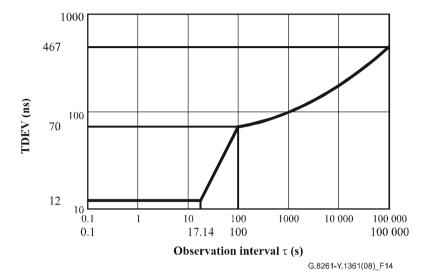
Figure 14 – Network limit for wander (TDEV) at synchronous equipment clock Option 1 interfaces
