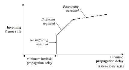
Figure I.2 – Variation of input stage delay with loading
