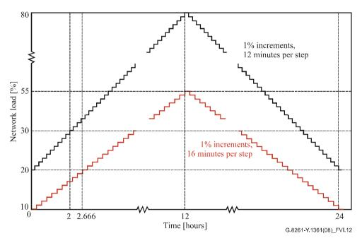
Figure VI.12 – Slow network load modulation for two-way
