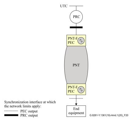
NOTE – The PEC is the PNT-F clock that is relevant in this model. The deployment of other clocks in the network (e.g. deployment of part of the PNT segment based on EEC and part on PEC) is for further study.
