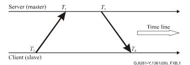
Figure XII.1 – Notion of time-stamps in packet exchange between a server and a client
