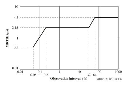
Figure 9 – Deployment Case 1: 2048 kbit/s interface wander budget
