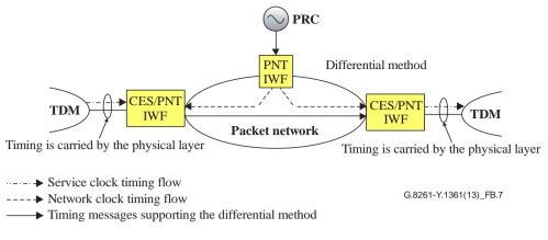
Figure B.7 – Example on timing recovery based on differential method
