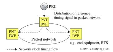
Figure B.9 – Reference timing distribution between IWF PNT
