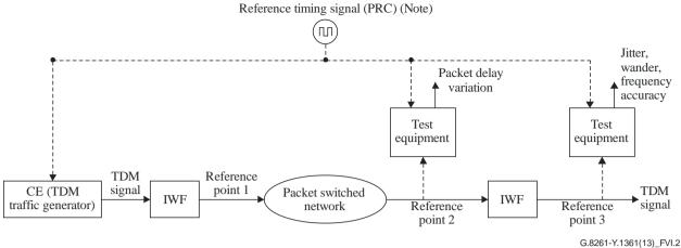
NOTE - The reference timing signal (PRC) is used to represent the TDM service clock.
