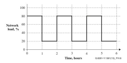
Figure VI.6 – Sudden network disturbance load modulation
