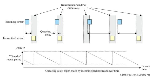
Figure 20-21 – Systematic delay variation caused by network with timeslots
