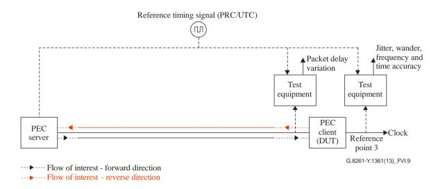
Figure VI.9 – Two-way baseline test topology
