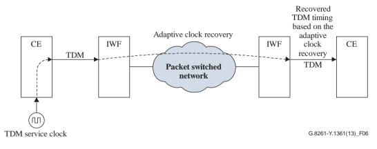
Figure 6 – Example of adaptive method
