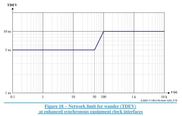
The minimum measurement period for TDEV is twelve times the maximum observation interval ( $T = 12\tau$ ).
