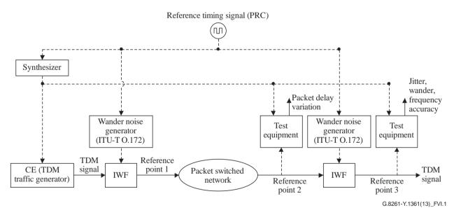
Figure VI.1 – Measurement reference points in the differential clock recovery method
