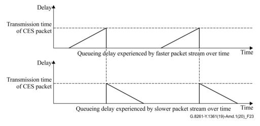
Figure <u>22-23</u> – Delay profile experienced by beating packet streams
