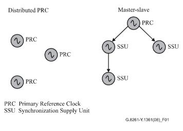
**Figure 1 – Distributed PRC and master-slave methods**
