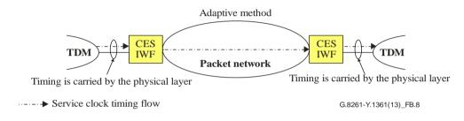
Figure B.8 – Example on timing recovery based on adaptive method
