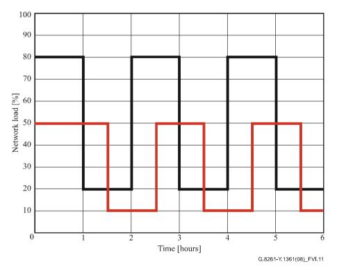
Figure VI.11 – Sudden network disturbance load modulation for 2-way
