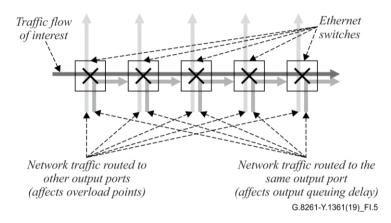
Figure I.5 – Data flows within an Ethernet network
