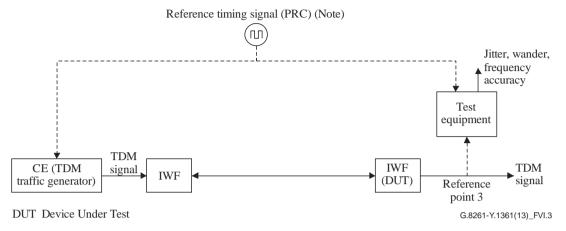
NOTE - The reference timing signal (PRC) is used to represent the TDM service clock.
