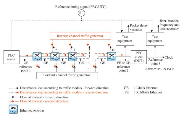
Figure VI.10 – Performance test topology for testing two-way protocols
