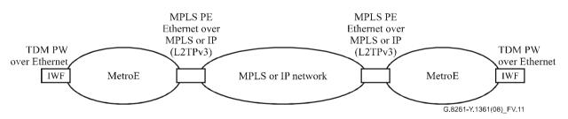
Figure V.11 – Ethernet over MPLS or IP network
