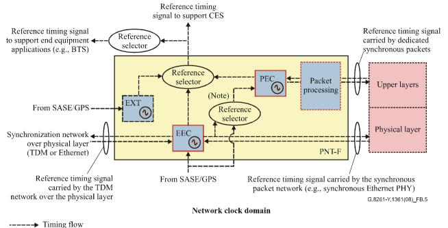
NOTE - Reference timing signal to support timing generation towards the packet side.
