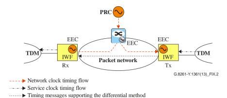
Figure IX.2 – Example of differential method using common reference
