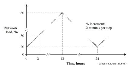
Figure VI.7 – Slow network load modulation
