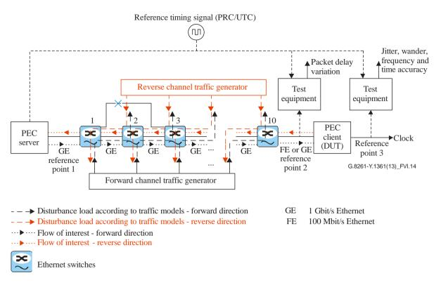
Figure VI.14 – Details of Test Case 17
