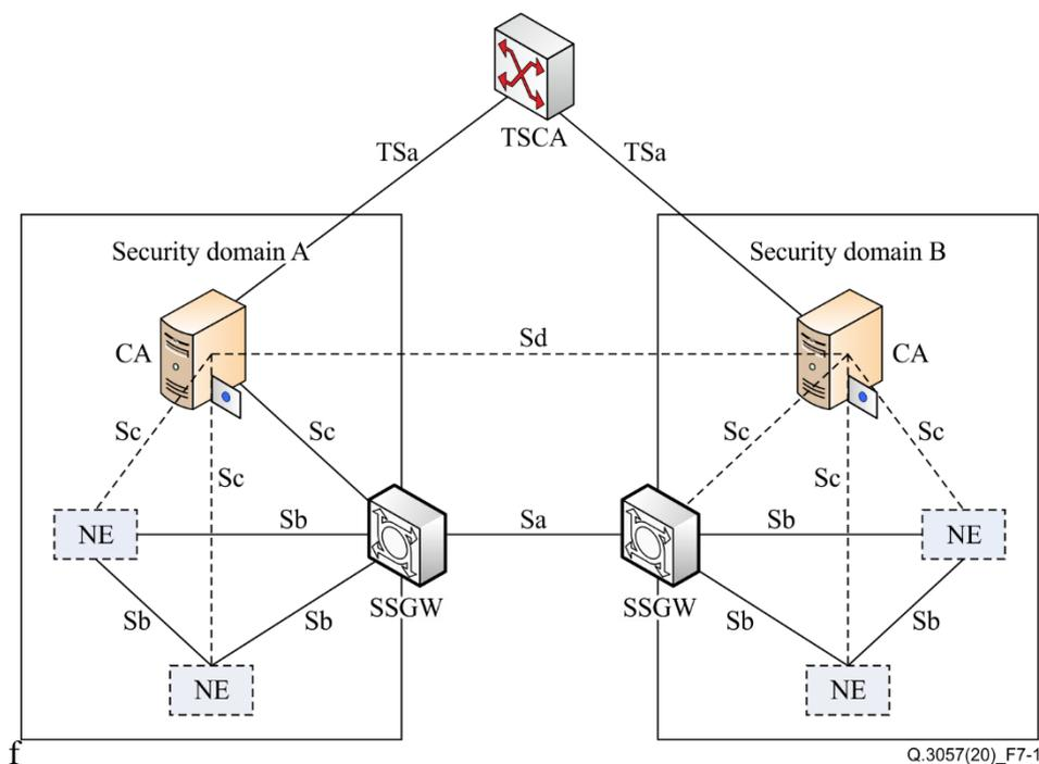
**Figure 7-1 – Reference architecture of interconnection between trustable network entities**
