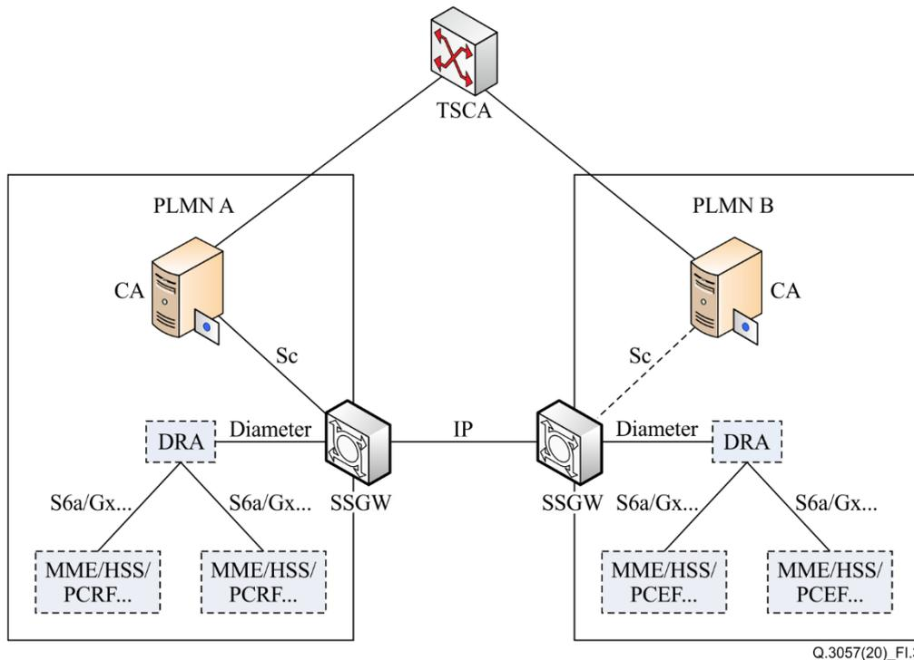
**Figure I.3 – Security Diameter transaction architecture**
