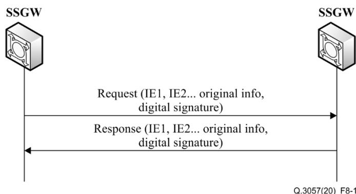
**Figure 8-1 – Information flow between SSGWs in different security domains**
