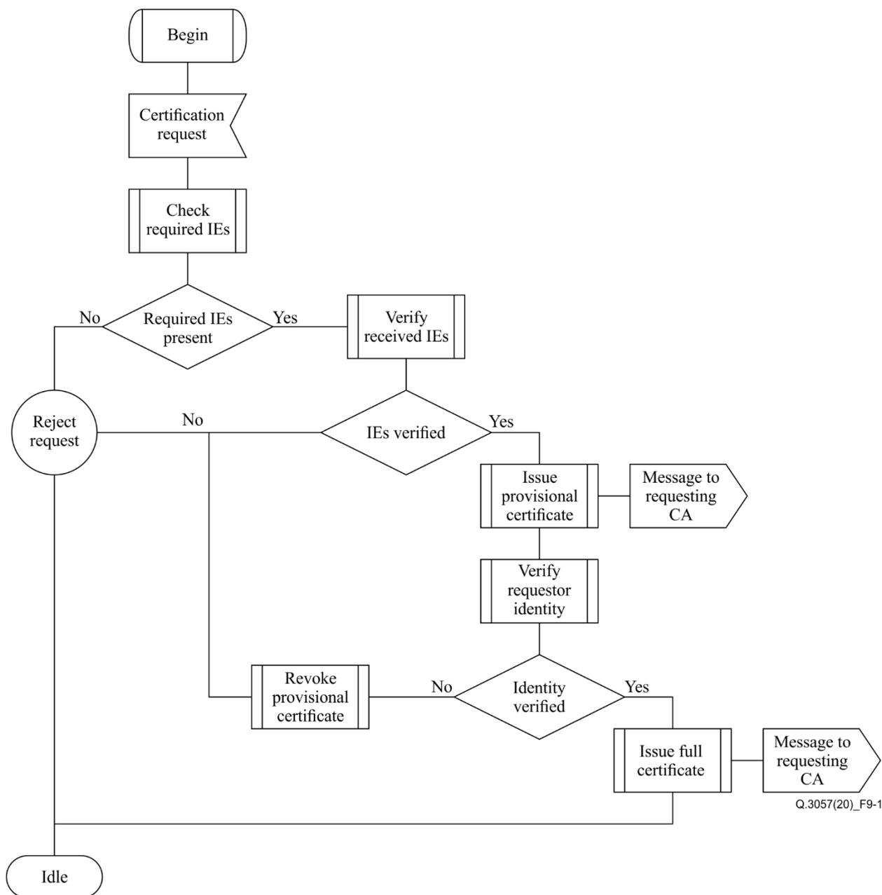
**Figure 9-1 – signalling procedures of TSCA**
