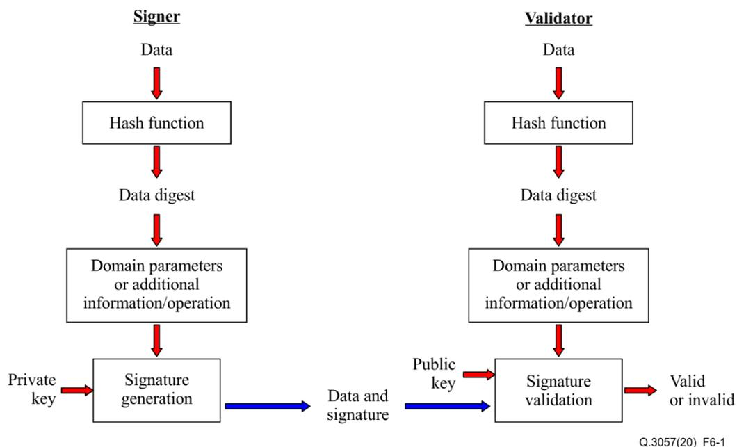
**Figure 6-1 – PKI digital signature verification process [ITU-T X.509]**
