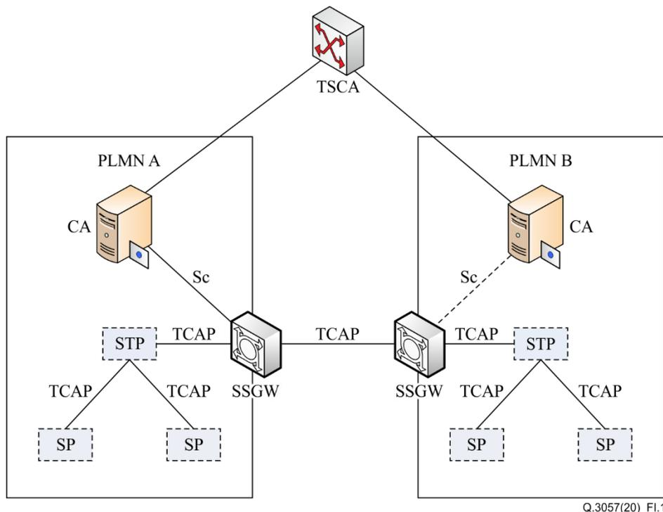
**Figure I.1 – Security TCAP transaction architecture**
