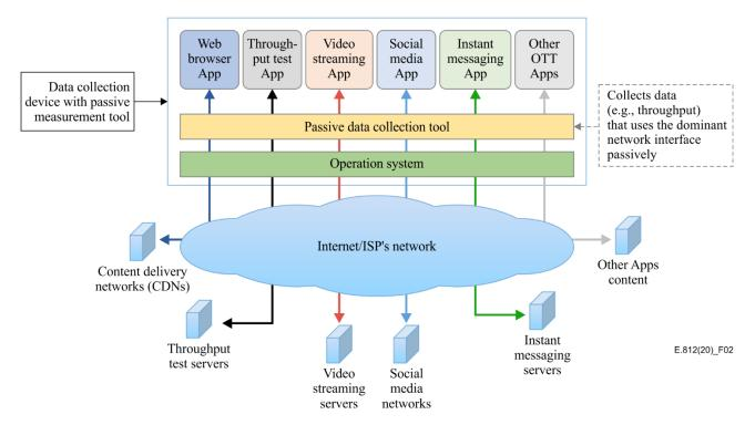
**Figure 2 – Example of passive data collection on mobile network**
