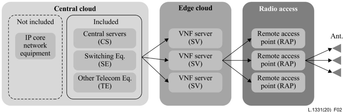
**Figure 2 – Generic CRAN architecture layout**
