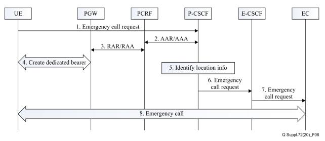
Figure 6 – Signalling procedure for LTE access
