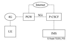
Figure 2 – UE accesses an IMS network via LTE access
