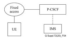
Figure 4 – UE accesses an IMS network via fixed access
