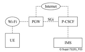
Figure 3 – UE accesses an IMS network via Wi-Fi access
