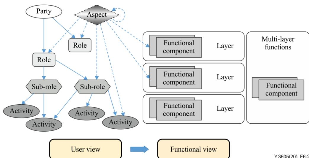
**Figure 6-2 – Transition from user view to functional view [ITU-T Y.3502]**
