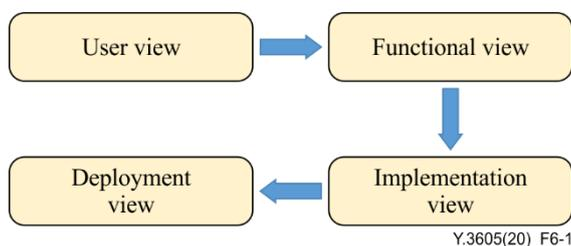
**Figure 6-1 – Transformations between architectural views [ITU-T Y.3502]**
