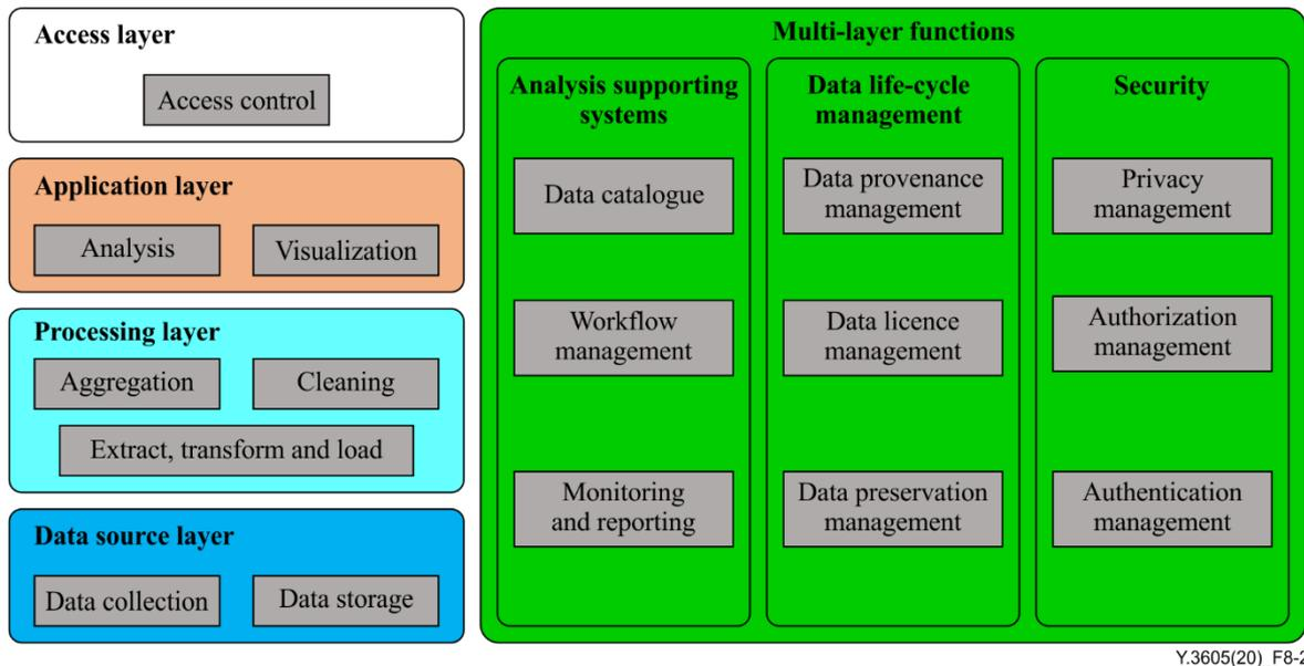
**Figure 8-2 – Big data functional components**
