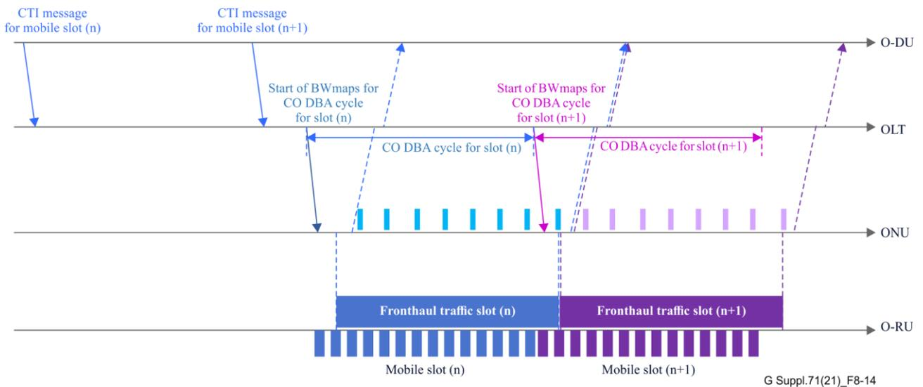
**Figure 8-14 – 1 CO DBA cycle per reported time interval**
