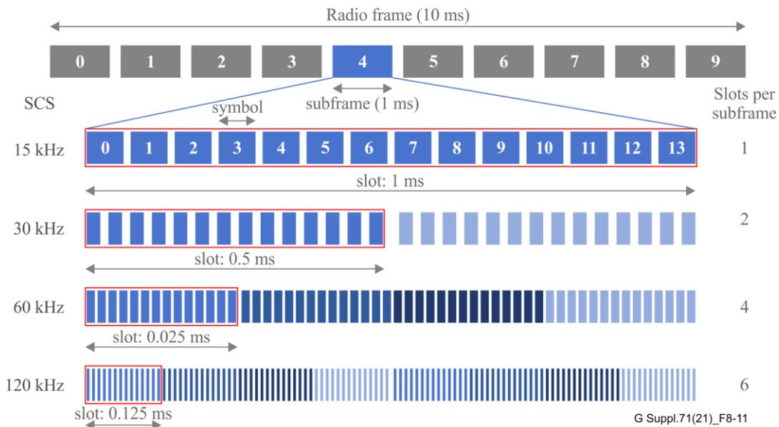
**Figure 8-11 – Time structures in RAN (sub-6 GHz) [b-NGMN Verticals]**
