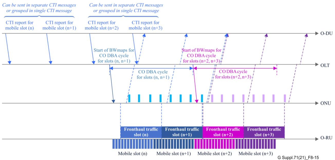
**Figure 8-15 – Multiple reported time intervals per CO DBA cycle**
