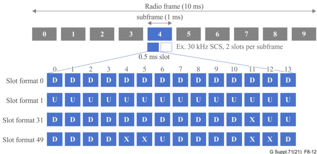
**Figure 8-12 – Dynamic slot configurations in 5G TDD: D-downstream symbol, U-upstream symbol, X-Flexible symbol: U,D or guard period (GP)**
