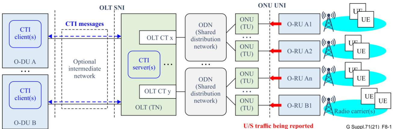
**Figure 8-1 – Transport of mobile fronthaul with CTI**
