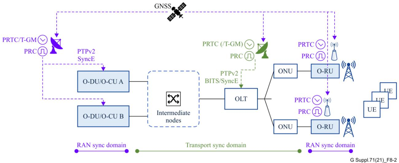
**Figure 8-2 – Access to common time of day by separate GNSS inputs (no explicit synchronization between RAN and transport domains)**
