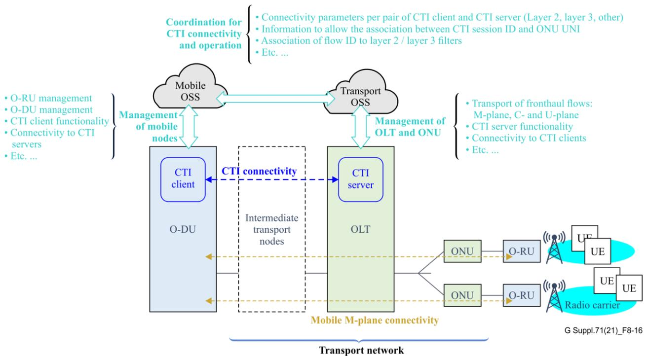
**Figure 8-16 – Mobile and transport OSS for management of CTI connectivity and CTI functionality**
