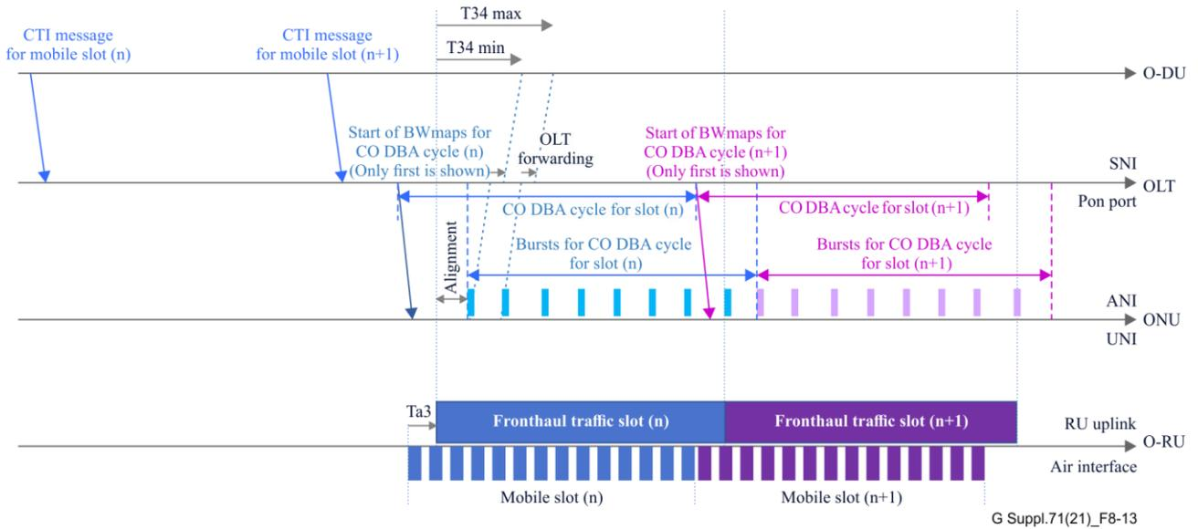
**Figure 8-13 – Alignment of CO DBA cycles with mobile slot boundaries at O-RU uplink**
