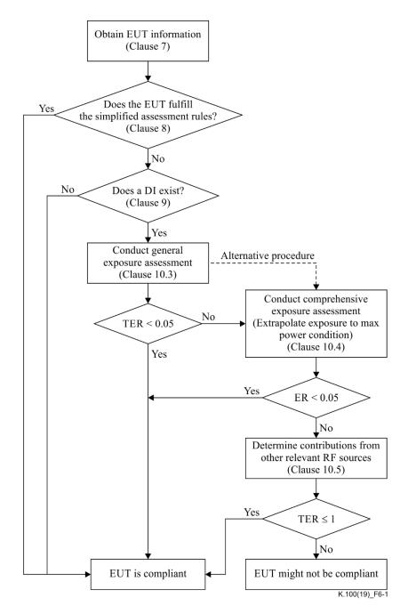
Figure 6-1 – Flowchart describing the measurement procedure specified in this Recommendation
