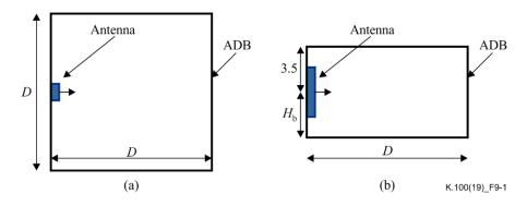
Figure 9-1 – a) Top-view of the square-shaped assessment domain boundary (ADB) with side length D.
