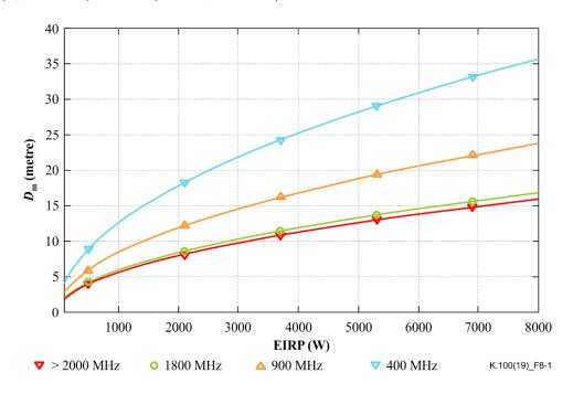
Figure  $8-1-D_m$  as a function of the equivalent isotropically radiated power obtained from Equations 8-1 to 8-3
