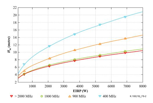
Figure 8-2 –  $H_m$  as a function of the equivalent isotropically radiated power obtained from Equations 8-1 to 8-3 based on a conservative choice of antenna parameters:  $\pi/12$  half-power beamwidth  $(\theta_{bw})$ ,  $\pi/12$  antenna downtilt  $(\alpha$ , electrical and mechanical) and side lobe suppression  $(A_{sl})$  of 0.05.  $H_m$  will decrease by decreasing  $\theta_{bw}$ ,  $\alpha$  and the side lobe suppression
