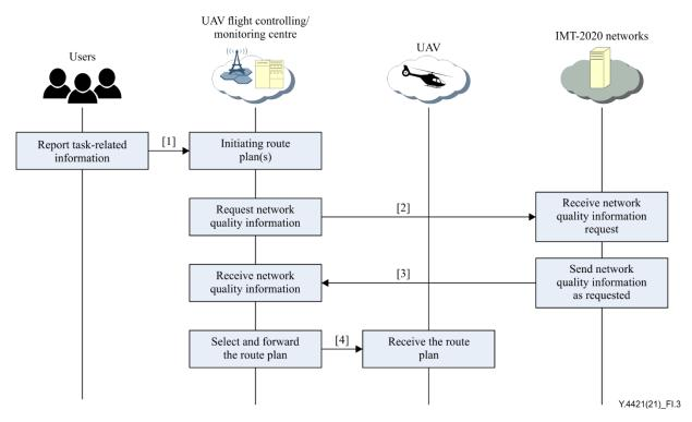
Figure I.3 – UAV route planning based on IMT-2020 networks
