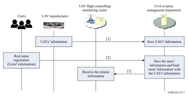
Figure I.1 – The UAV and the user are registered based on IMT-2020 networks
