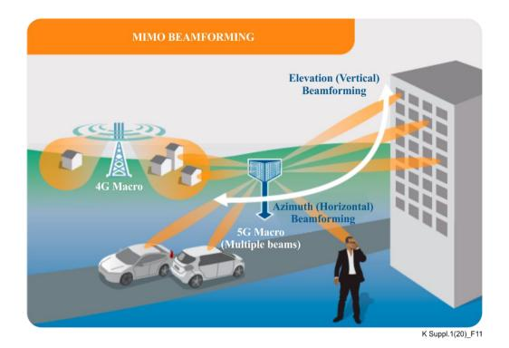
Figure 11 – MIMO beamforming
