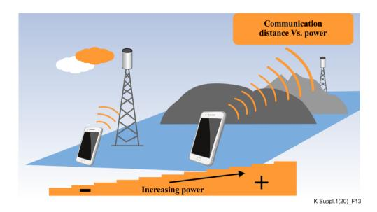
Figure 13 – Distance from base station and increasing phone power (the + indicates higher power from a mobile phone is required)
