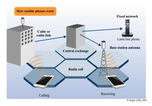
Figure 4 – How mobiles devices and base stations work
