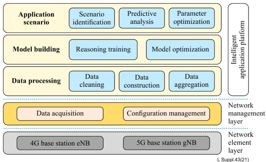
**Figure 2 – Overall architecture of a 5G intelligent energy-saving network**
