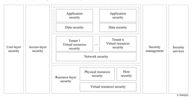
Figure 6-1 – Virtualization container security framework
