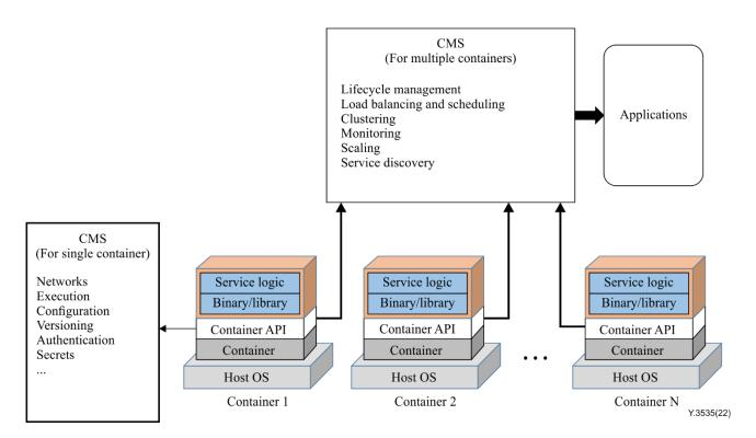
Figure 6-4 – Concept of the container management system
