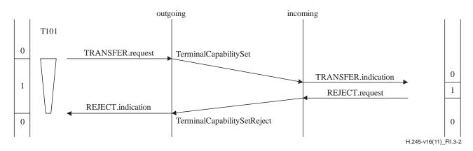
Figure II.3-2 – Capability exchange with rejection from peer incoming CESE user
