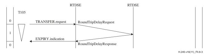
Figure II.8-3 – Round-trip delay determination procedure with timer T105 expiry
