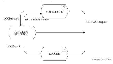
Figure C.43 – State transition diagram for sequence of primitives at outgoing MLSE
