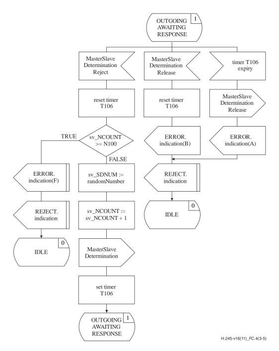
Figure C.4 – MSDSE SDL (sheet 3 of 5)
