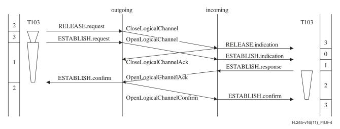
Figure II.9-4 – Bidirectional logical channel release followed by immediate re-establishment
