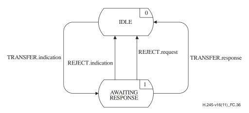
Figure C.36 – State transition diagram for sequence of primitives at incoming MRSE
