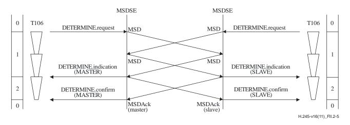
Figure II.2-5 – Master-slave determination – Simultaneous determination but with the first attempt returning an indeterminate result
