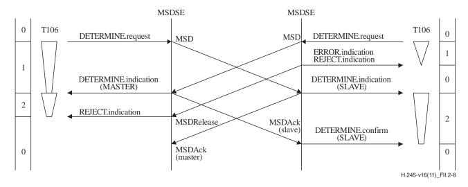
Figure II.2-8 – Master-slave determination – Simultaneous determination procedures with timer T106 expiry at slave
