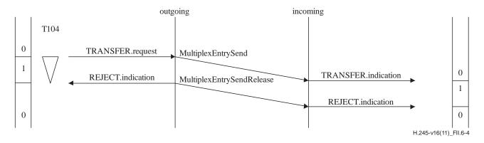
Figure II.6-4 – Multiplex table send request with timer T104 expiry
