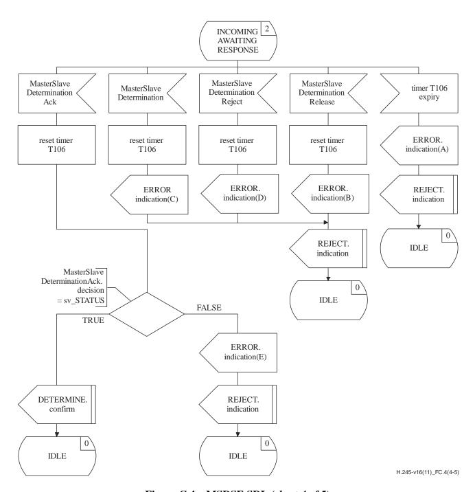
Figure C.4 – MSDSE SDL (sheet 4 of 5)
