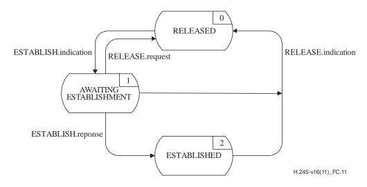
Figure C.11 – State transition diagram for sequence of primitives at incoming LCSE
