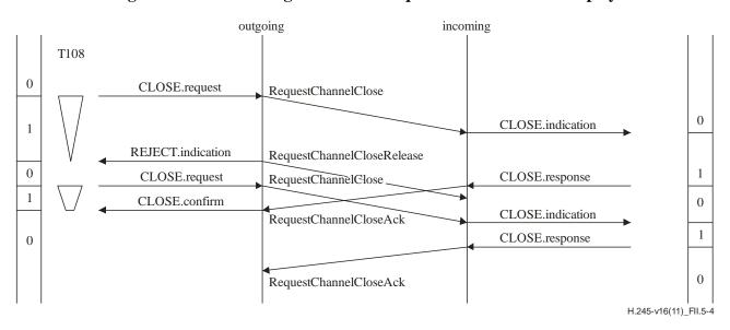
NOTE - The Close channel request is confirmed on reception of the first RequestChannelClose message.
