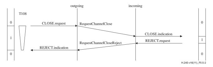
Figure II.5-2 – Close logical channel request with rejection from peer incoming CLCSE user
