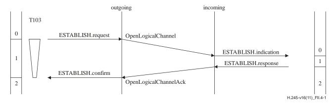
Figure II.4-1 – Logical channel establishment
