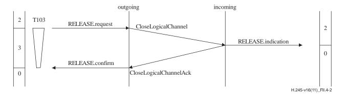
Figure II.4-2 – Logical channel release
