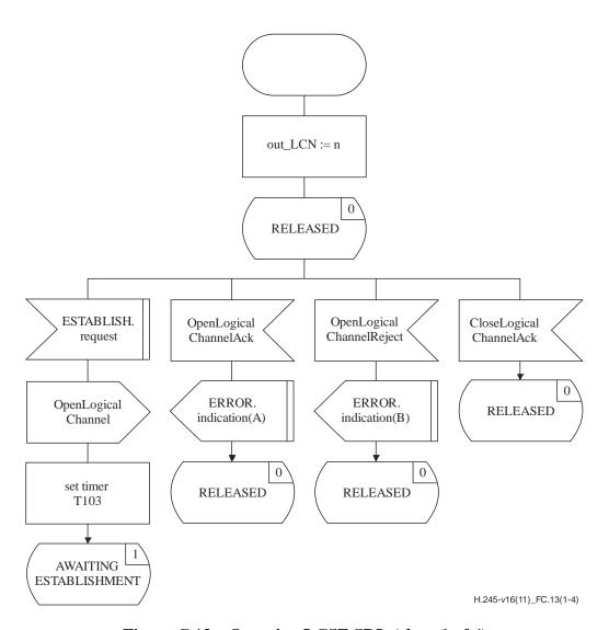
Figure C.13 – Outgoing LCSE SDL (sheet 1 of 4)
