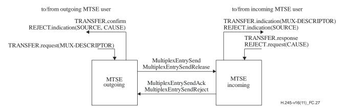
Figure C.27 – Primitives and messages in the Multiplex Table Signalling Entity
