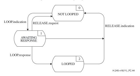
Figure C.44 – State transition diagram for sequence of primitives at incoming MLSE
