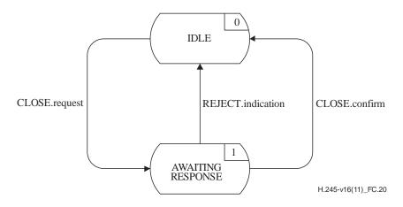
Figure C.20 – State transition diagram for sequence of primitives at outgoing CLCSE
