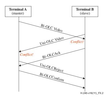
Figure X.2 – Master proposes bidirectional OLC and slave proposes unidirectional OLC
