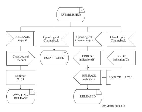
Figure C.13 – Outgoing LCSE SDL (sheet 3 of 4)
