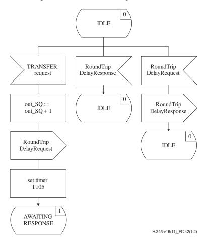
Figure C.42 – RTDSE SDL (sheet 1 of 2)
