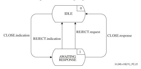
Figure C.21 – State transition diagram for sequence of primitives at incoming CLCSE
