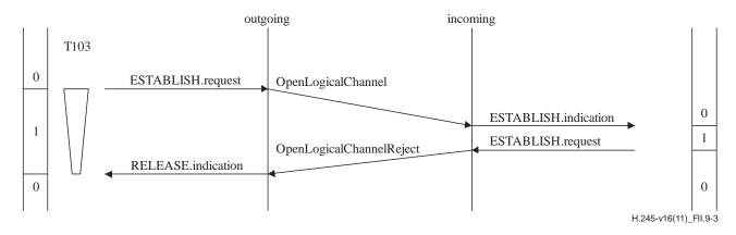
Figure II.9-3 – Bidirectional logical channel establishment rejection by peer B-LCSE user
