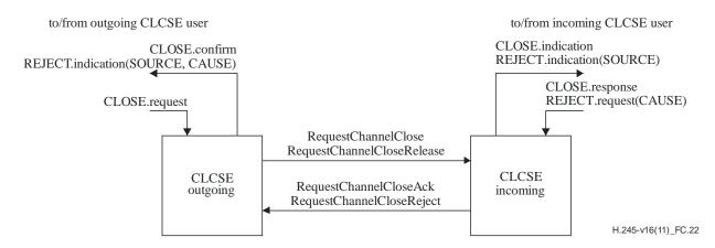
Figure C.22 – Primitives and messages in the Close Logical Channel Signalling Entity
