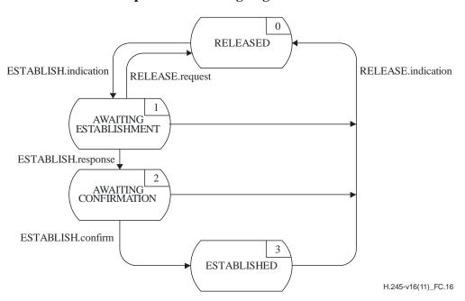
Figure C.16 – State transition diagram for sequence of primitives at incoming B-LCSE
