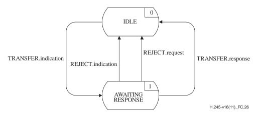
Figure C.26 – State transition diagram for sequence of primitives at incoming MTSE
