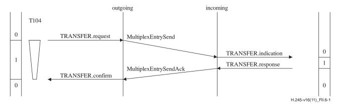
Figure II.6-1 – Successful multiplex table send request
