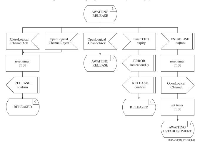
Figure C.18 – Outgoing B-LCSE SDL (sheet 4 of 4)
