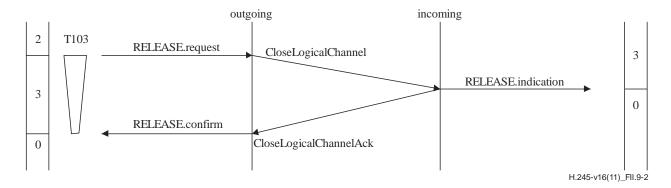
Figure II.9-2 – Bidirectional logical channel release
