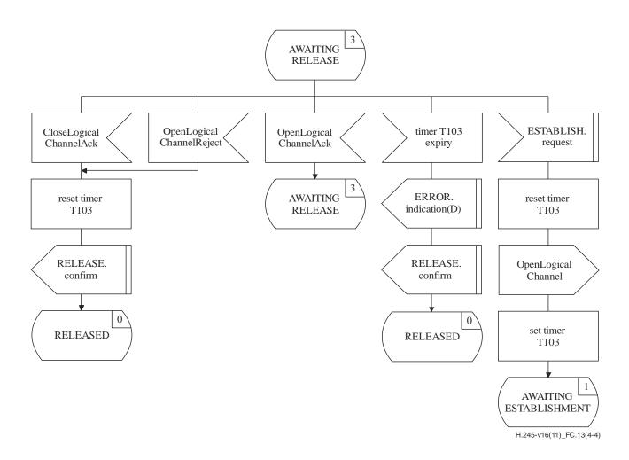
Figure C.13 – Outgoing LCSE SDL (sheet 4 of 4)
