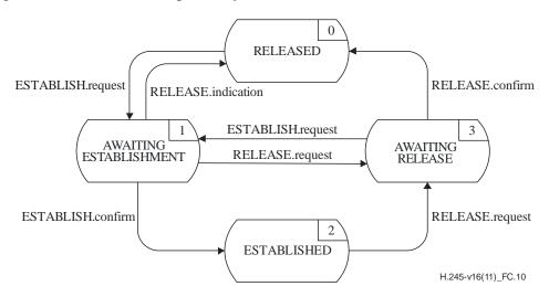
Figure C.10 – State transition diagram for sequence of primitives at outgoing LCSE
