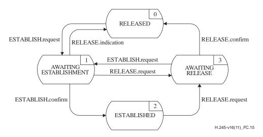
Figure C.15 – State transition diagram for sequence of primitives at outgoing B-LCSE
