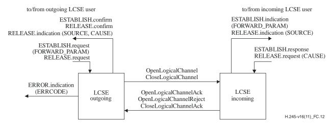
Figure C.12 – Primitives and messages in the Logical Channel Signalling Entity
