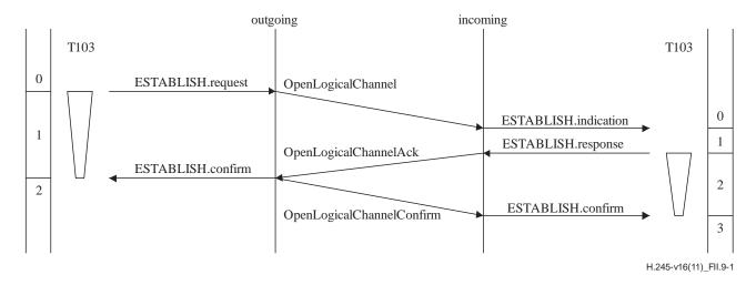
Figure II.9-1 – Bidirectional logical channel establishment
