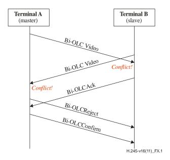
Figure X.1 – Both terminals use bidirectional OLC
