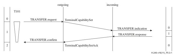
Figure II.3-1 – Capability exchange with acceptance from the peer incoming CESE user
