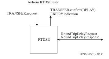
Figure C.41 – Primitives and messages in the RTDSE
