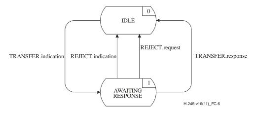
Figure C.6 – State transition diagram for sequence of primitives at incoming CESE
