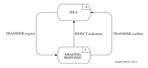
Figure C.5 – State transition diagram for sequence of primitives at outgoing CESE
