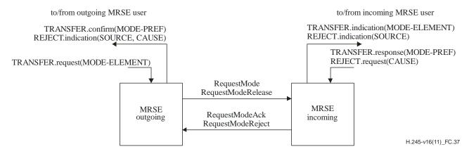
Figure C.37 – Primitives and messages in the Mode Request Signalling Entity
