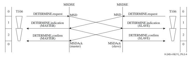
Figure II.2-4 – Master-slave determination – Simultaneous determination
