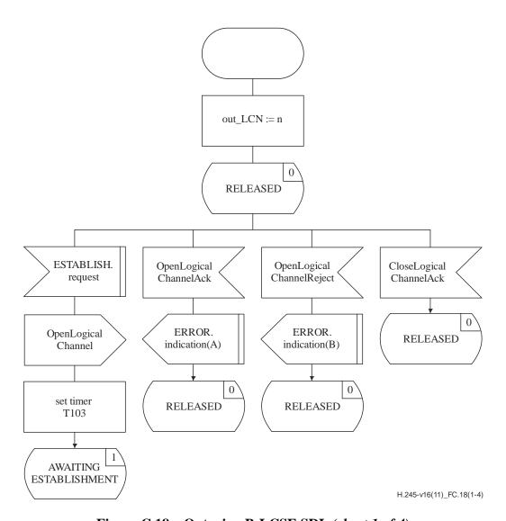
Figure C.18 – Outgoing B-LCSE SDL (sheet 1 of 4)
