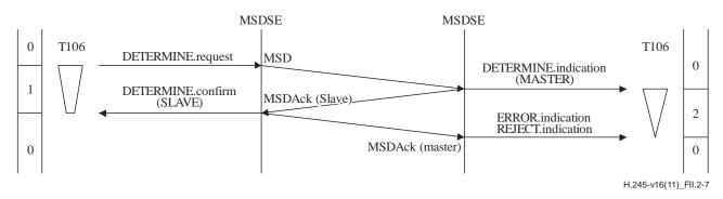
Figure II.2-7 – Master-slave determination – Remote timer T106 expiry with master at remote end
