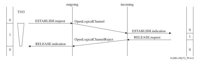
Figure II.4-3 – Logical channel establishment rejection by peer LCSE user
