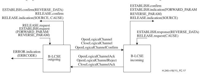
Figure C.17 – Primitives and messages in the bidirectional Logical Channel Signalling Entity
