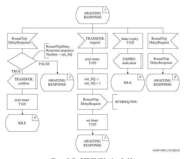
Figure C.42 – RTDSE SDL (sheet 2 of 2)
