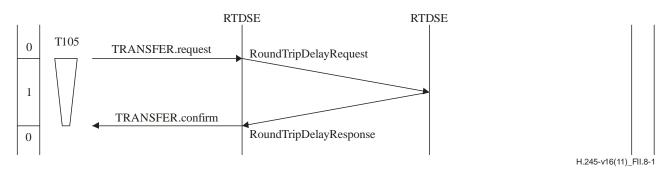
Figure II.8-1 – Round-trip delay determination procedure
