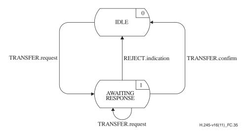
Figure C.35 – State transition diagram for sequence of primitives at outgoing MRSE
