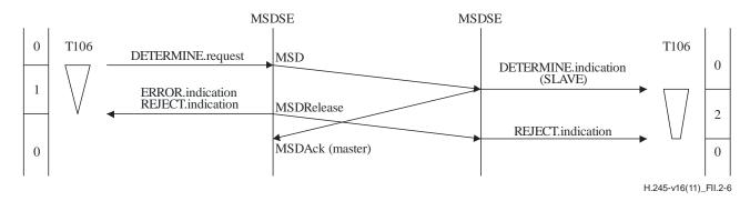
Figure II.2-6 – Master-slave determination – Local timer T106 expiry with slave at remote end
