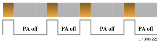
Figure 3 – Illustration of time-domain energy saving: During symbols with no information to transmit, the PA is deactivated
