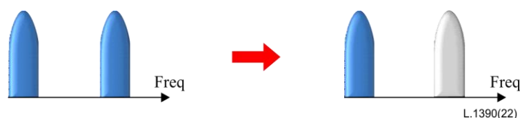
Figure 5 – Illustration of large-scale frequency-domain energy saving, carrier shutdown: One of the two carriers is shutdown, and the related radio unit is deactivated to save energy
