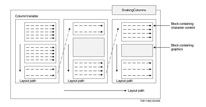
$\label{eq:FIGURE-8/T.506} FIGURE\ 8/T.506$  Example of the layout of a snaking columns frame
