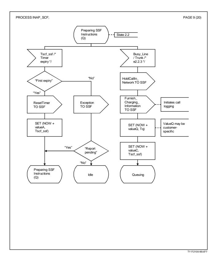
FIGURE A.3/Q.1218 (sheet 9 of 20) SDL for SCF-FSM
