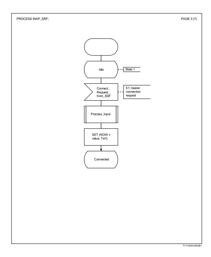
FIGURE A.4/Q.1218 (sheet 3 of 7) SDL for SRF-FSM
