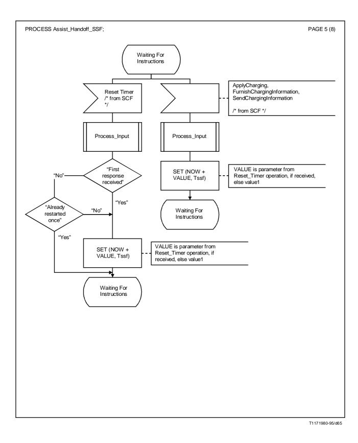
FIGURE A.2/Q.1218 (sheet 5 of 8) SDL for assist/handoff SSF-FSM
