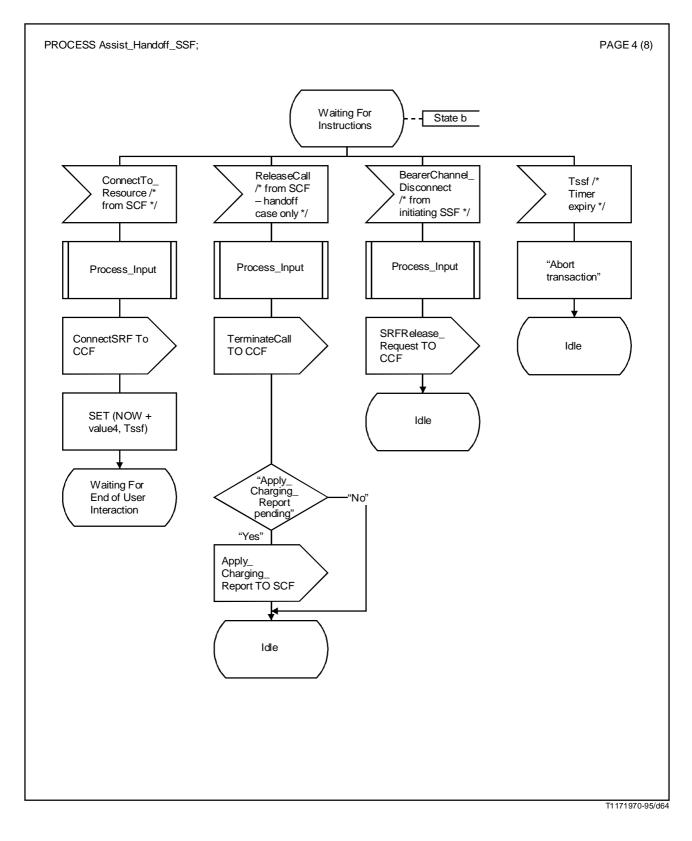
FIGURE A.2/Q.1218 (sheet 4 of 8) SDL for assist/handoff SSF-FSM
