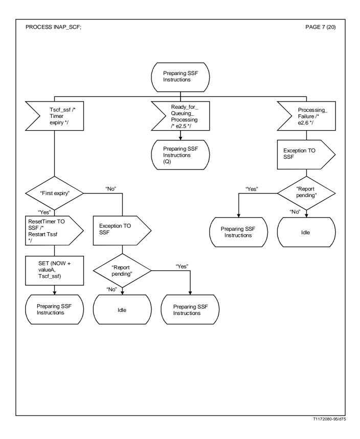
FIGURE A.3/Q.1218 (sheet 7 of 20) SDL for SCF-FSM
