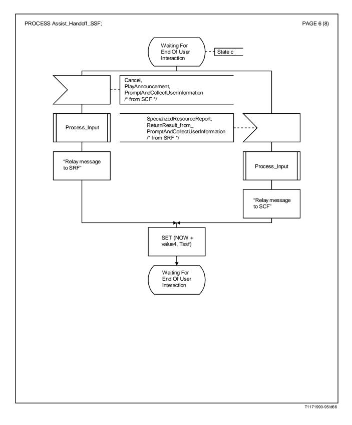
FIGURE A.2/Q.1218 (sheet 6 of 8) SDL for assist/handoff SSF-FSM
