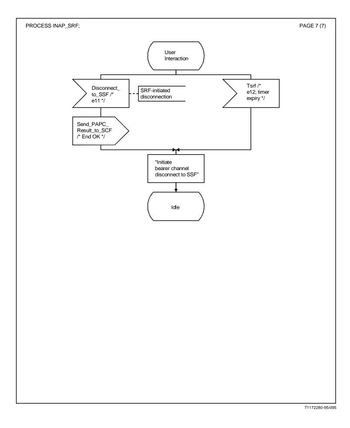
FIGURE A.4/Q.1218 (sheet 7 of 7) SDL for SRF-FSM
