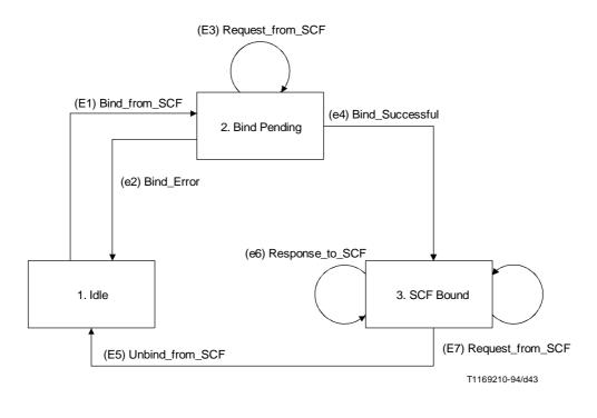
FIGURE 42/Q.1218 The SDF-FSM
