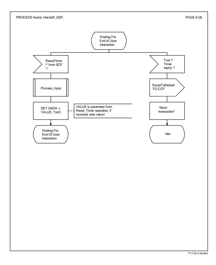
FIGURE A.2/Q.1218 (sheet 8 of 8) SDL for assist/handoff SSF-FSM
