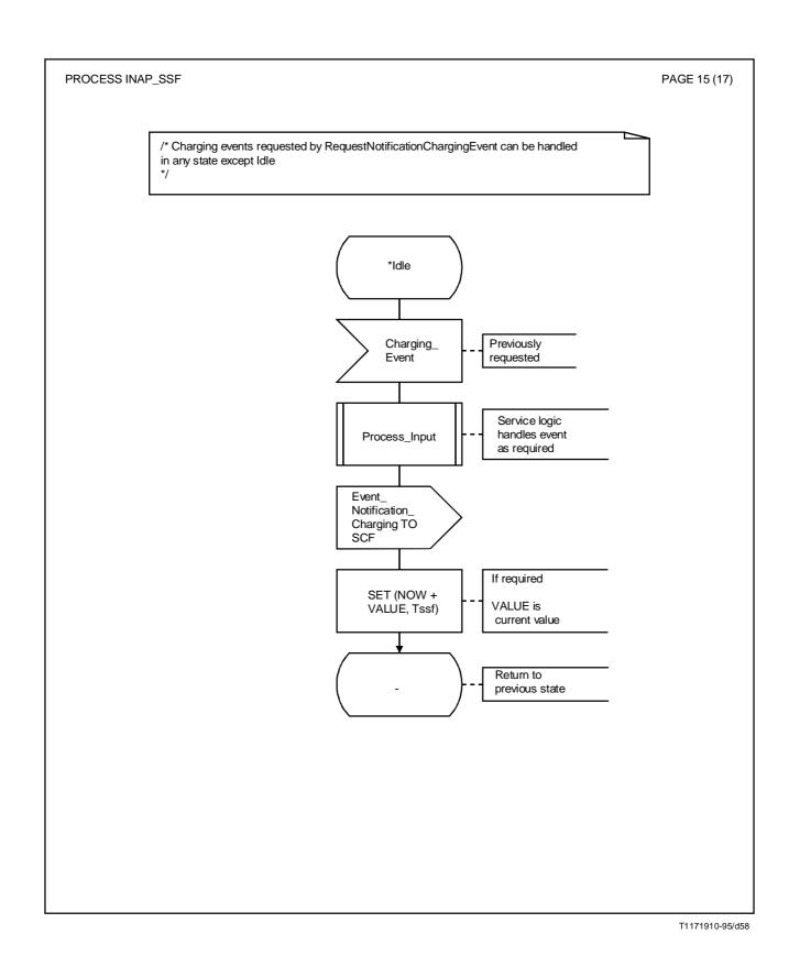
FIGURE A. 1/Q. 1218 (sheet 15 of 17) SDL for SSF-FSM
