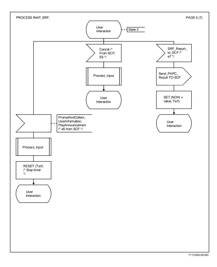
FIGURE A.4/Q.1218 (sheet 5 of 7) SDL for SRF-FSM
