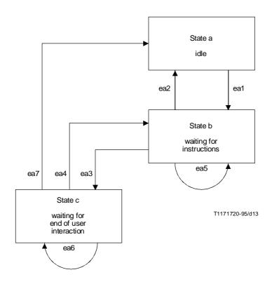
FIGURE 13/Q.1218 Assisting/Handoff SSF finite state machine
