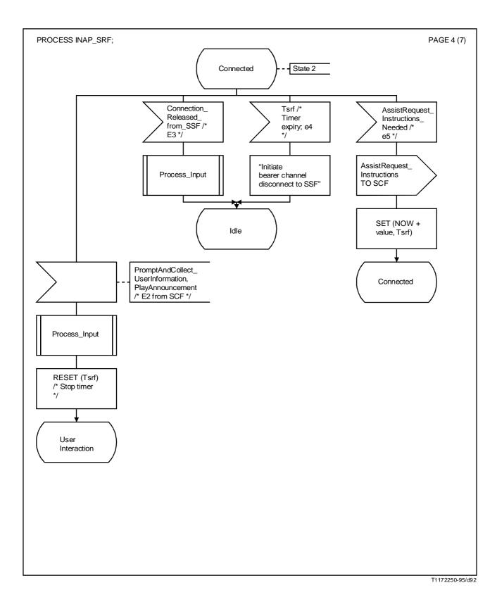
FIGURE A.4/Q.1218 (sheet 4 of 7) SDL for SRF-FSM
