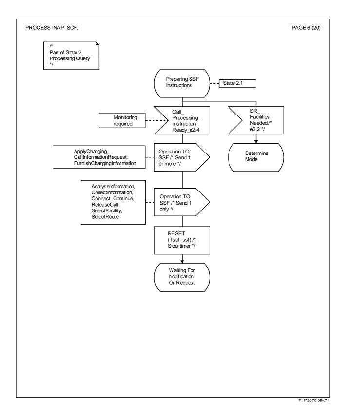
FIGURE A.3/Q.1218 (sheet 6 of 20) SDL for SCF-FSM
