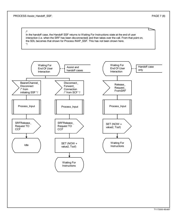
FIGURE A.2/Q.1218 (sheet 7 of 8) SDL for assist/handoff SSF-FSM
