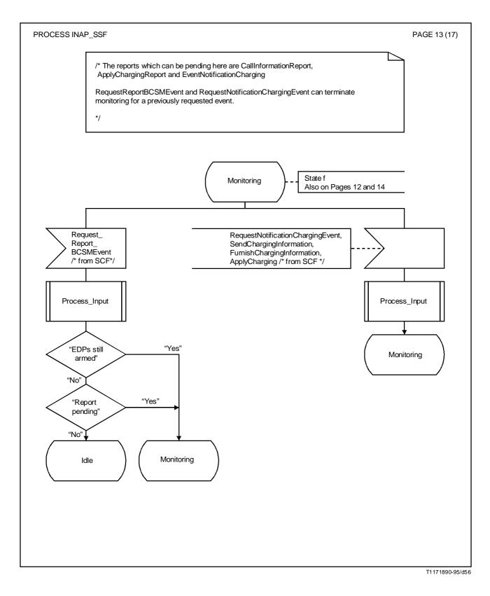
FIGURE A.1/Q.1218 (sheet 13 of 17) SDL for SSF-FSM
