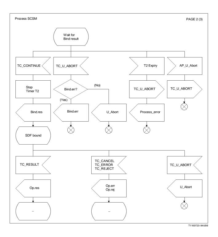
FIGURE B.2/Q.1218 (sheet 2 of 3) SCSM
