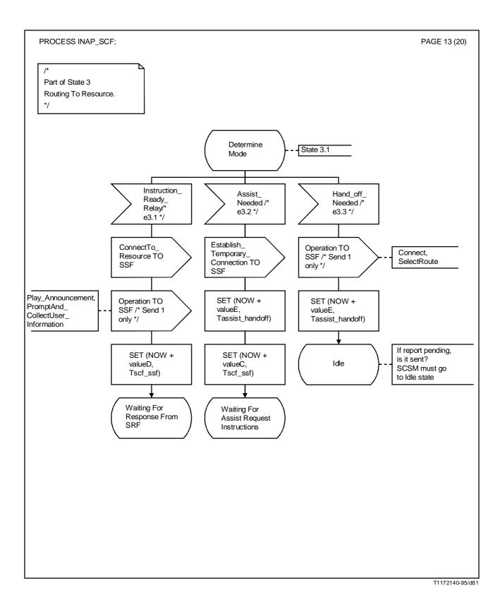
FIGURE A.3/Q.1218 (sheet 13 of 20) SDL for SCF-FSM
