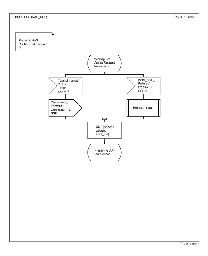
FIGURE A.3/Q.1218 (sheet 16 of 20) SDL for SCF-FSM
