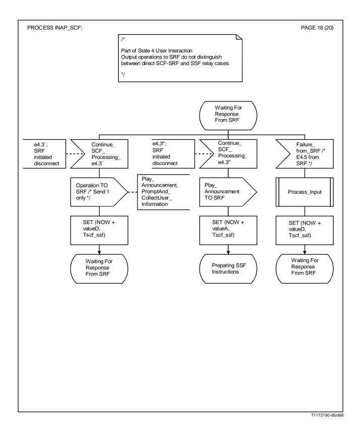
FIGURE A.3/Q.1218 (sheet 18 of 20) SDL for SCF-FSM
