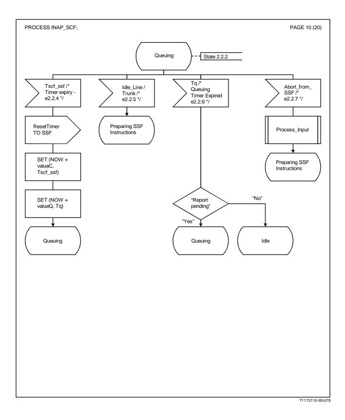
FIGURE A.3/Q.1218 (sheet 10 of 20) SDL for SCF-FSM
