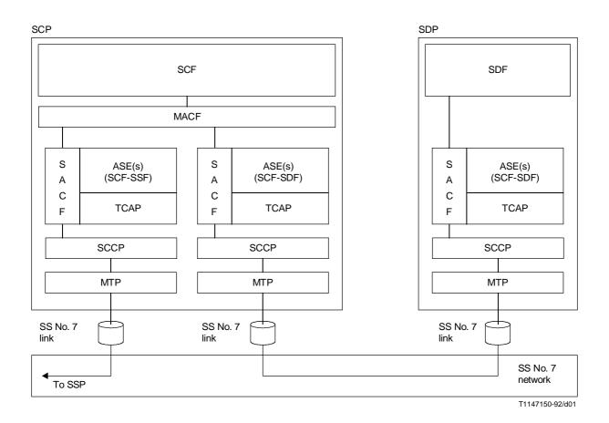
FIGURE 1/Q.1218 Physical interface between SCP and SDP
