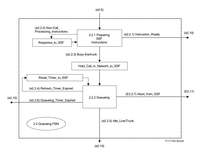
FIGURE 20/Q.1218 Partial expansion of the State 2 FSM as related to queueing
