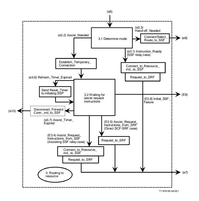
FIGURE 21/Q.1218 The State 3 FSM
