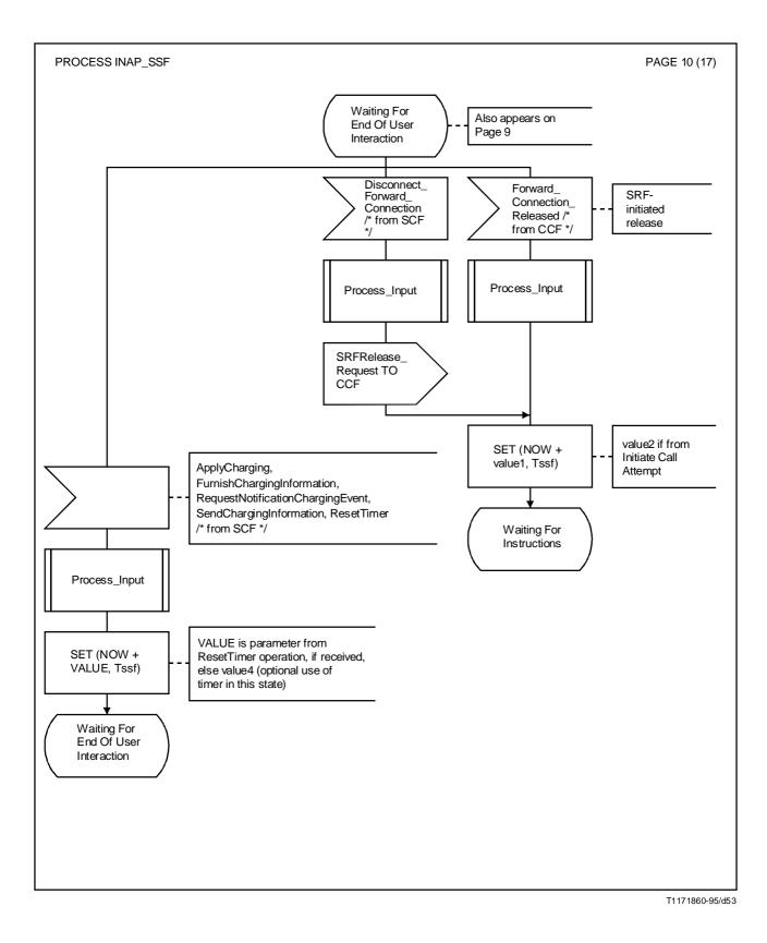
FIGURE A.1/Q.1218 (sheet 10 of 17) SDL for SSF-FSM
