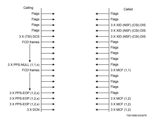
The document being transmitted consists of several partial pages with no errors on the received document.
