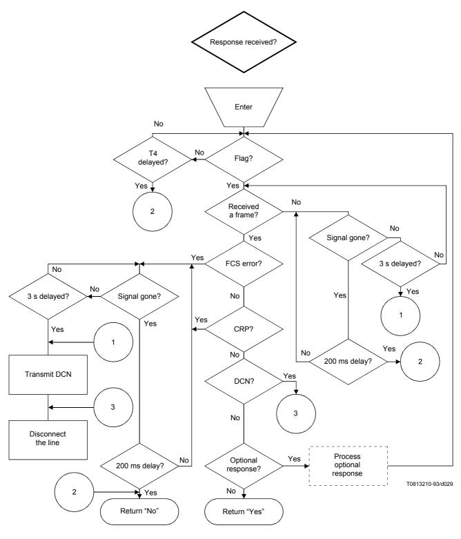
T4 =  $4.5 \text{ s} \pm 15\%$  for manual units T4 =  $3.0 \text{ s} \pm 15\%$  for automatic units
