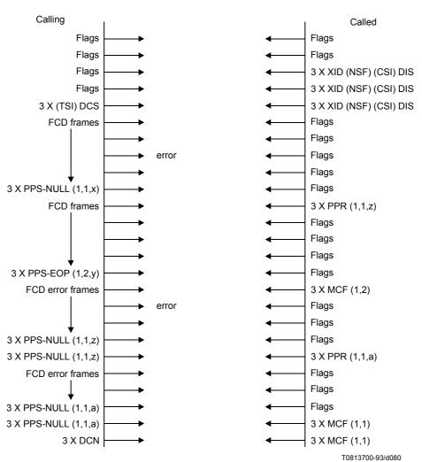
The document being transmitted consists of several partial pages with errors on the received document and errors on the corrections.
