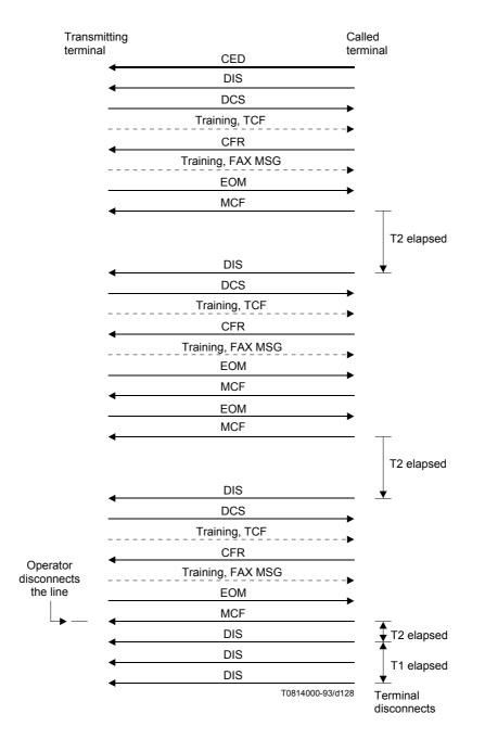
*Example 2* A single page transmitter wishing to transmit to an auto answer terminal: example of EOM.
