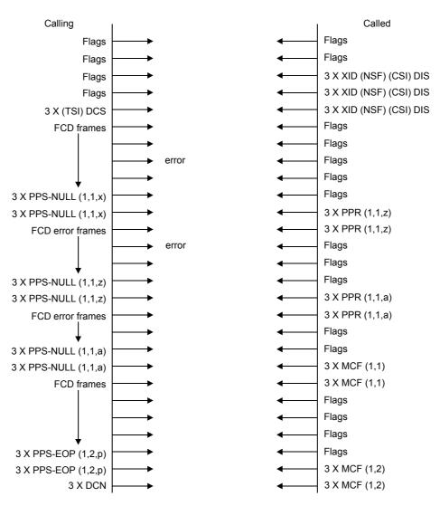
The document being transmitted consists of several partial pages with errors on the received document and errors on the corrections.
