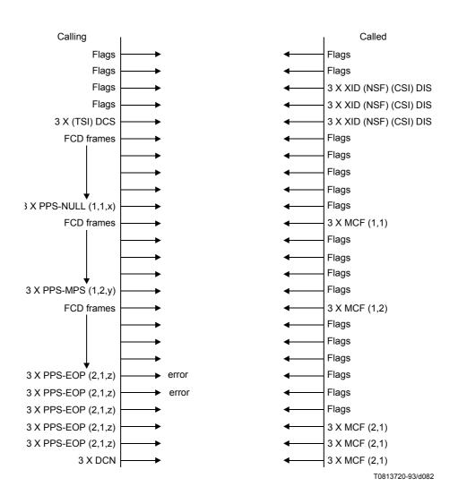
The document being transmitted consists of several partial pages with errors on the last post-message command.
