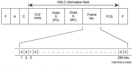
Octet 5(PC) Page counter (8 bits: modulo 256) Octet 6(BC) Block counter (8 bits: modulo 256)
