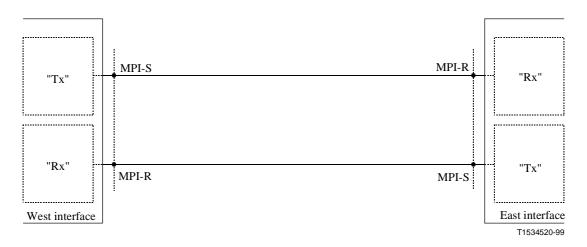
Figure 2/G.664 – Reference configuration for description of ALS capability
