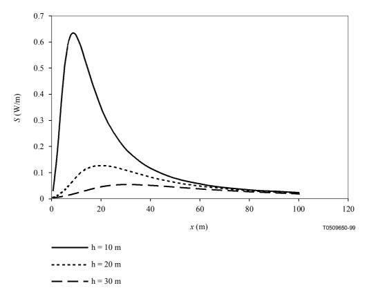
Figure II.2/K.52 – Power density at the ground level vs. distance from the tower calculated for the example II.1
