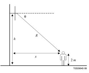
Figure II.1/K.52 – Sample configuration for calculating exposure at ground level
