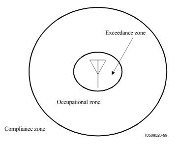
Figure 1/K.52 – Figurative illustration of exposure zones
