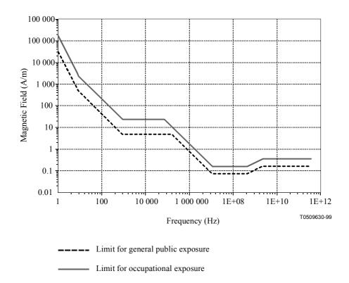
Figure I.2/K.52 – ICNIRP reference limits for magnetic field strength
