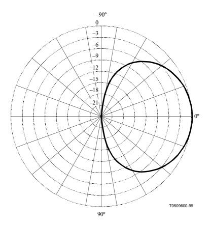
Figure B.6/K.52 – Vertical pattern for a half-wave dipole
