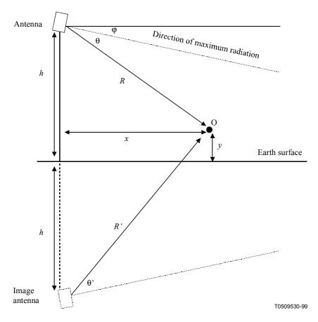
Figure 2/K.52 – Definition of distances and vertical angles
