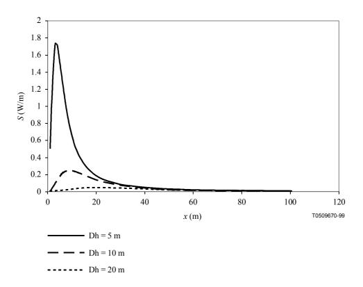
Figure II.4/K.52 – Power density at the ground level vs. distance from the tower calculated for the example II.2
