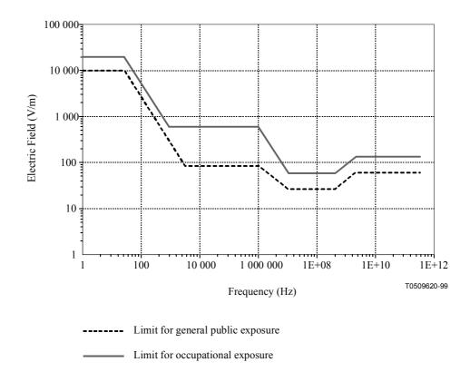
Figure I.1/K.52 – ICNIRP reference limits for electric field strength
